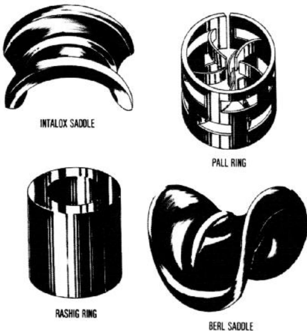
**Figure 6. Four common types of packing.**
