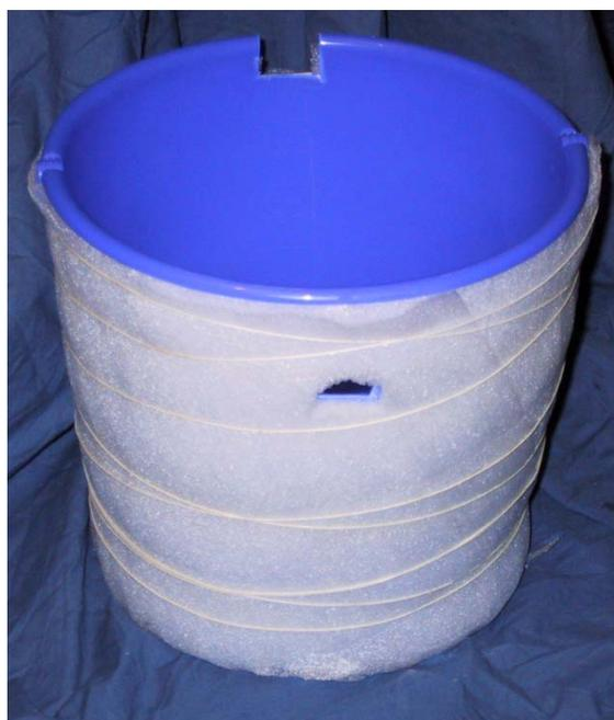
It is not difficult to insulate. Cut a strip of insulation making it 1 metre long and a bit wider than the vessel. (Roll out a length and cut off). Place it round the vessel and tie in place with cotton string. Cut off surplus insulation round the top and bottom of the vessel and cut out the holes. The insulation is very easy to cut so this is simple. Put on more layers and bind fast until you finally have a thickness of 10 mm or more. It's finished!
