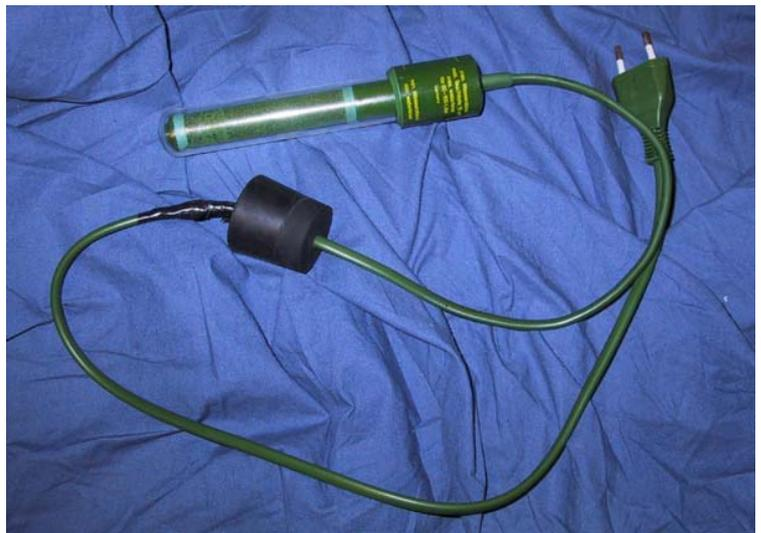
Unfortunately nearly all thermostats have a maximum setting of 32 degrees C. This heat is too low and it would take for ever to produce anything. A suitable temperature range for this unit is 45 – 52 degrees C. Buy an immersion heater with a thermostat that goes up to 55 degrees C.
