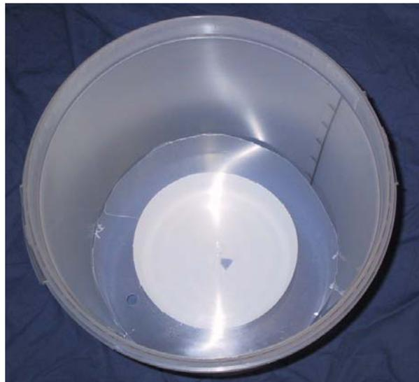
Here is a picture showing the container from the side with a glass disc. There should be 5 litres capacity for the alcohol in the bottom. As the fermenting vessel has volume graduation on the outside it is easy to see how high the disc should be placed.
