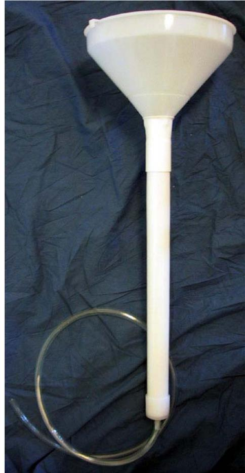
Some carbon brands are poorly washed at the factory, so pour 3-5 litres of hot water through the activated carbon before you purify the spirit so as to wash out the salts not wanted in the spirit. Also the cleaning function of the carbon is enhanced if it is wet. Wait an hour or preferably 24 hours after washing and then wash again with 2 litres of hot water. Then you only have to pour the spirit in the top. Discard the water that comes out first.
