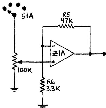
Fig. 5 -- Adjustable full-scale range.
