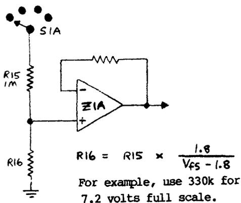
Fig. 4 -- Adding an input attenuator for high full-scale meters, such as voltmeters.
