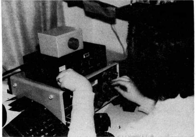
Fig. 1 — WB8TDA tunes her antenna with help from the ASWRI. The ASWRI sits atop, and monitors, a Ten Tec model 228 antenna tuner. It is best to do the initial tuning with the meter sensitivity at maximum, and the transmitter drive just high enough to reach the forward full-scale setting. Kitty also uses the ASWRI to tune her transmitter for peak output by setting the meter to read forward power at reduced sensitivity.
