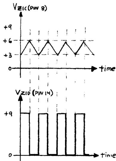
Fig. 11 — VCO waveforms for circuit in Fig. 10.
