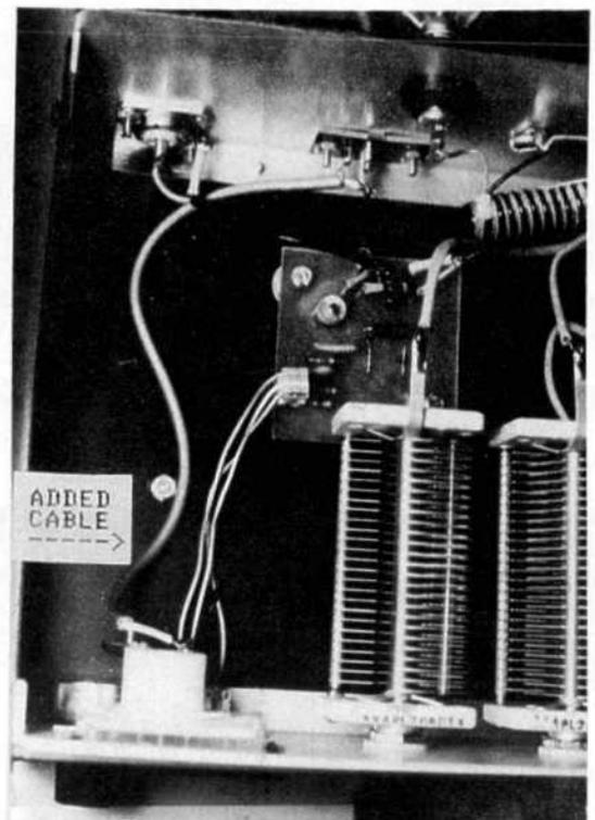
Fig. 9 — Adding meter output to the Ten Tec 228 antenna tuner.
