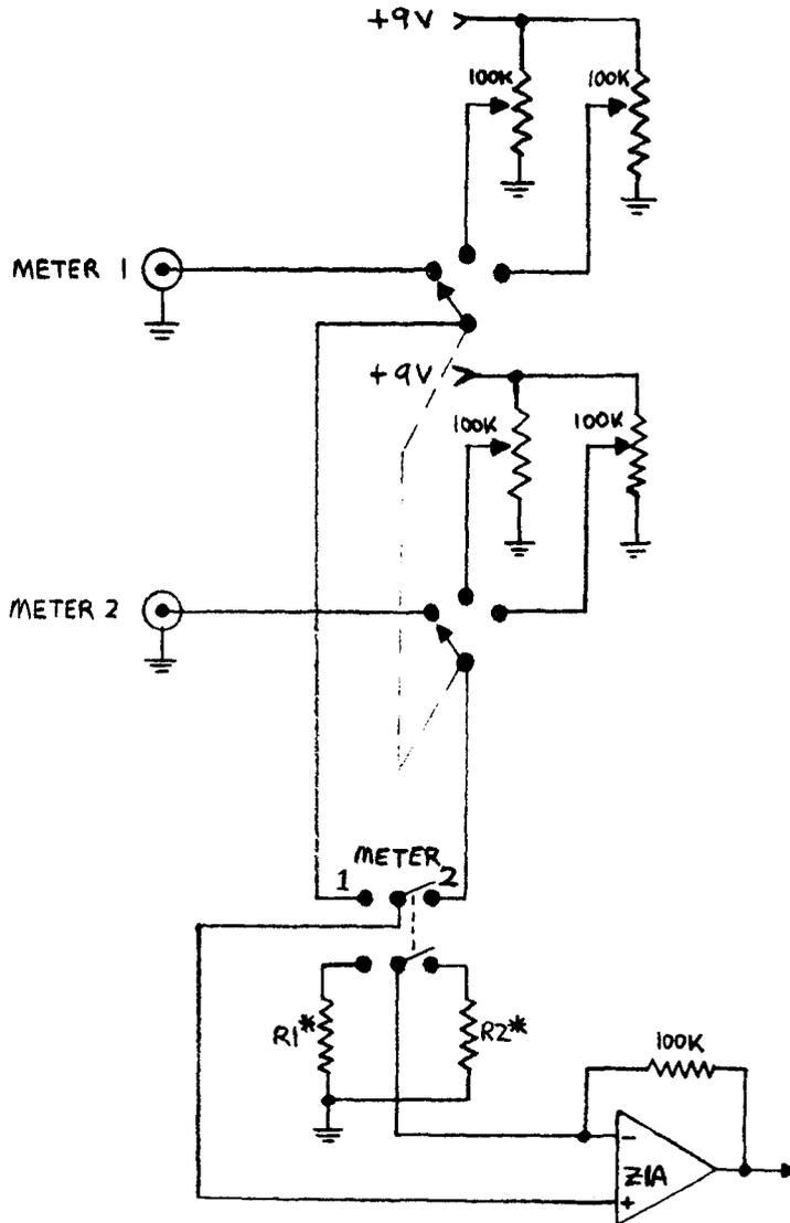
Fig. 12 -- Adapting the circuit to monitor multiple meters.
