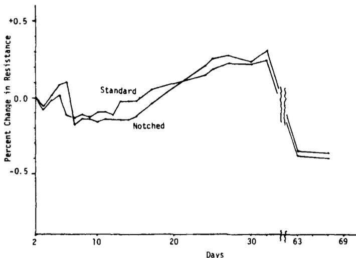
Fig. 1 -- Notched and standard resistors exposed to room air.
