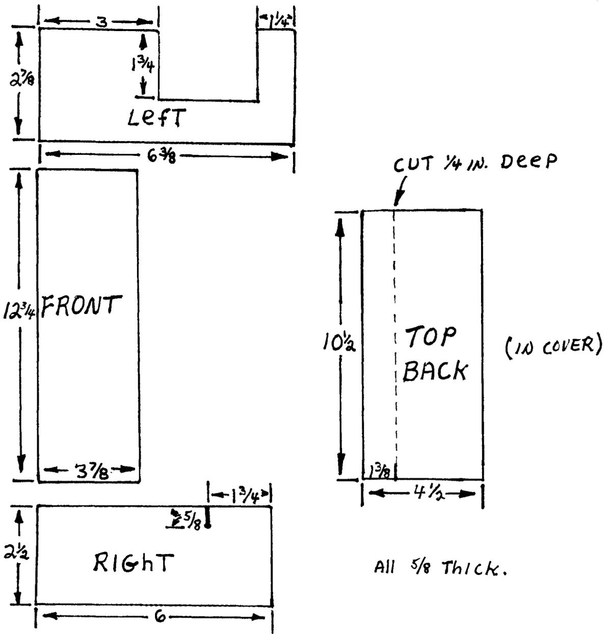
Fig. 1 — Dimensions for cutting the foam padding to be inserted in sections of the printer cover. All dimensions are in inches and the diagrams are not drawn to scale.
