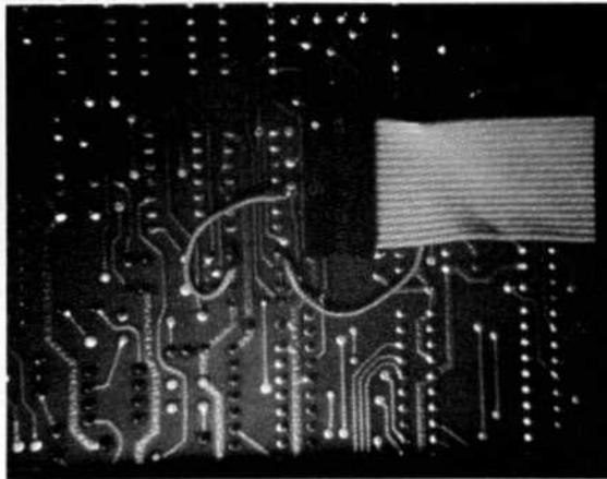
Photo 7 -- A close up of the added wiring to the RS-232-C board. See Fig. 2 also.
