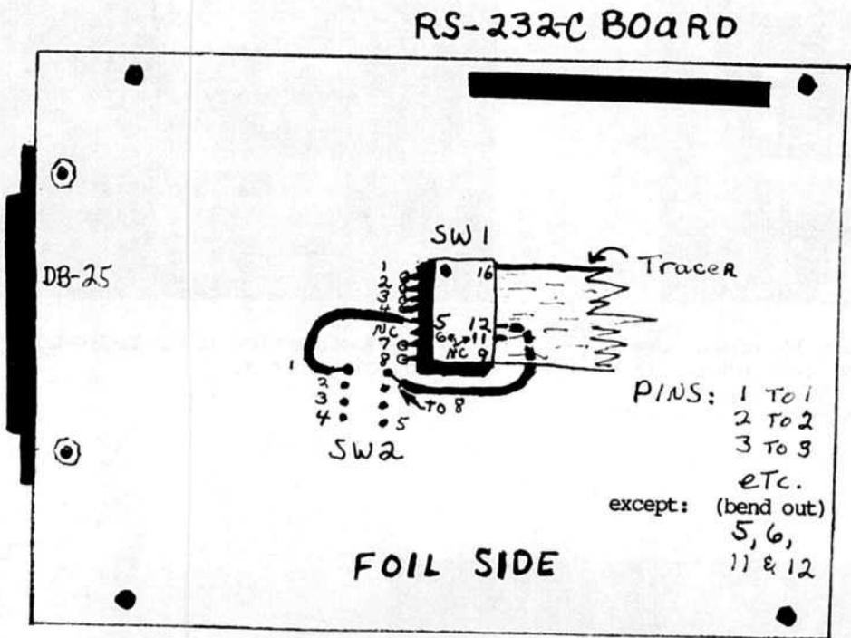
Fig. 2 -- The RS-232-C board showing pin connections.
