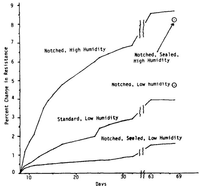
Fig. 2 -- Behavior of resistors exposed to high and low humidities.
