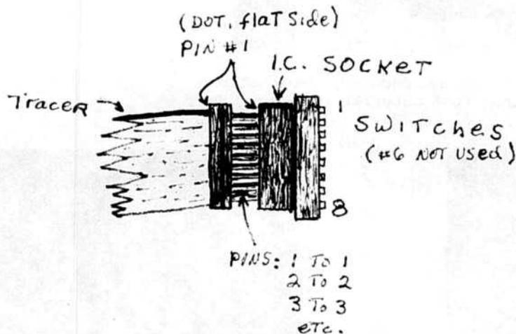
Fig. 3 -- A close up view showing the cable wiring.
