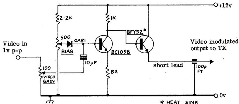
Fig 4 VIDEO MODULATOR FOR 2W TRANSMITTERS
