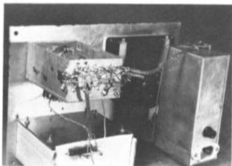
Fig. 11: Inside are 3 screened modules and a meter
