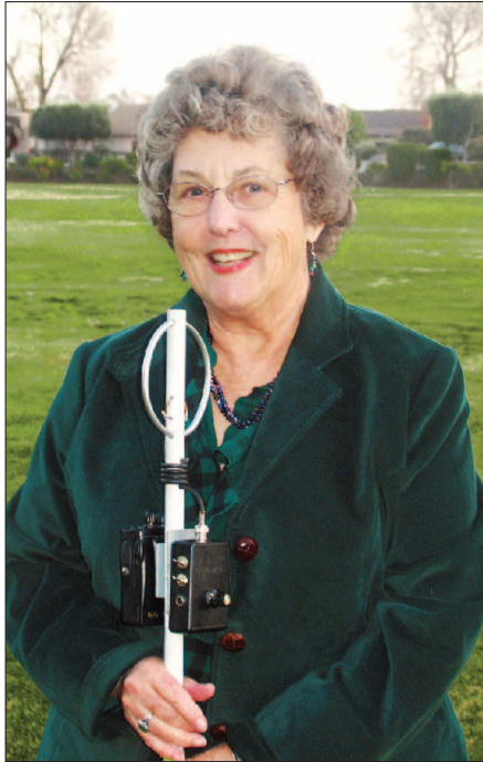
Figure 5 — Carol Adams, KG6VLG, demonstrating the use of body fade . Note the placement and orientation of the loop. She is facing the hidden transmitter.
