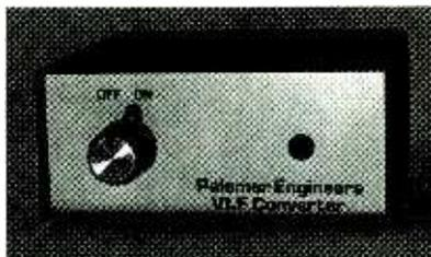
*The Palomar Engineers VLF Converter lets you receive the low bands for about \$80; all you need to receive WWVB and other low-frequency stations, along with the so-called 1750-meter experimenters' band, is a communications receiver and an antenna. Covering 10–500 kHz, the Model VLF-A converts VLF signals to the 80-meter amateur band, while the Model VLF-S converts signals to 4010–4500 kHz for general coverage SW receivers.*
