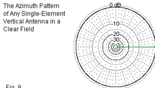
The performance of a basic vertical antenna will show itself almost completely in elevation patterns. We shall look at several dimensions of the vertical as we think of it as a multi-band antenna. We shall examine four main dimensions: the feedpoint position, the length, and the height above ground, and the ground itself. Together, these factors will form our basic performance expectations.
