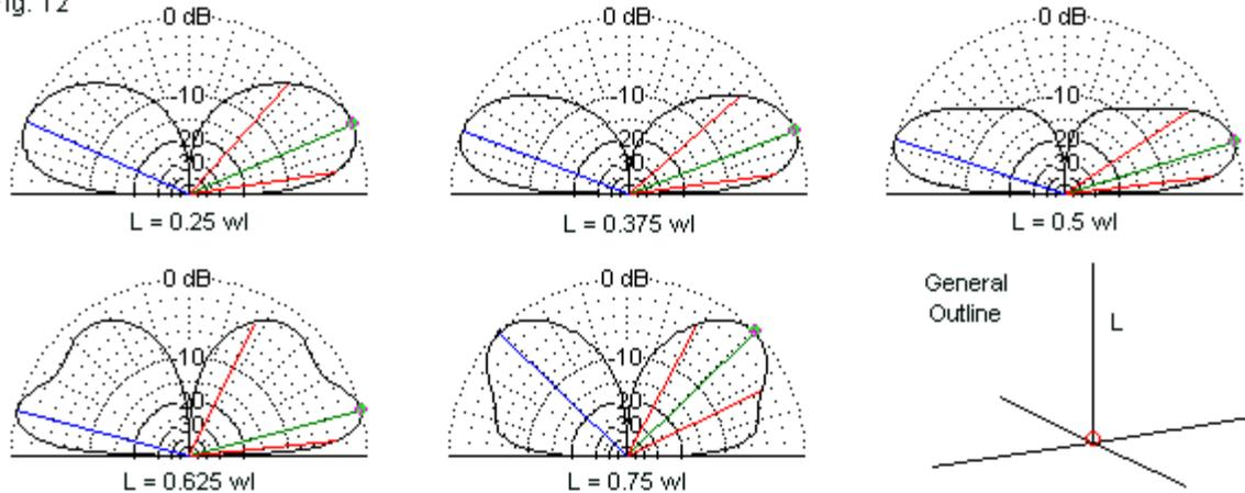
Elevation Patterns of a Monopole of Various Lengths
