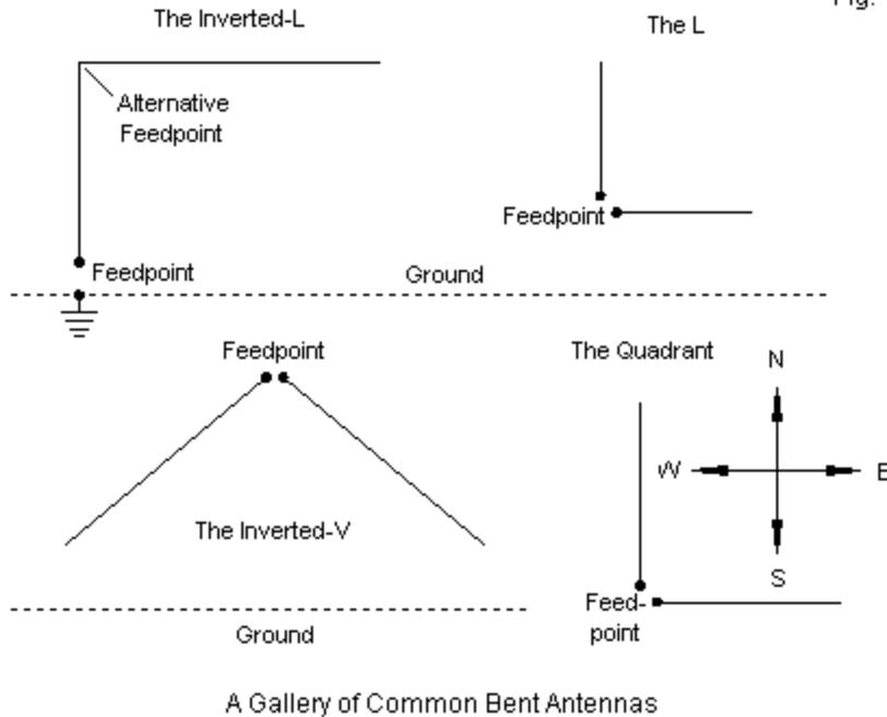
All of the antennas in **Fig. 19** are essentially the same antenna. If you bend a half-wavelength wire in the middle and keep the feedpoint there, then the resonant impedance—after pruning—drops from the typical dipole value of  $70 \Omega$  down to the  $50\text{-}\Omega$  vicinity. The only difference among the antennas in the sketch is the orientation of the wire around the bend. However, that difference makes a big difference in application.
