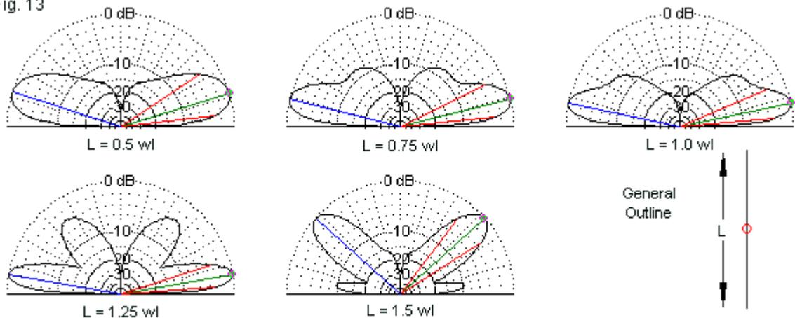
Elevation Patterns of a Vertical Dipole of Various Lengths
