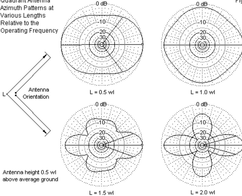
Although the quadrant multi-band doublet is not a true (unterminated) V-beam, the right-angle bend places it near the edge of that category, especially as the total length grows to 3 or 4  $\lambda$ . At longer lengths for each side of the center feedpoint, the antenna provides more consistent bi-directional performance than a straight doublet. Hence, the antenna may have more appeal than simply as a way to fit a horizontal antenna into limited yard space.
