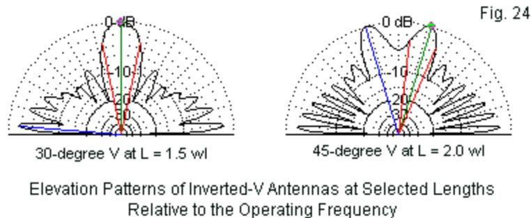
**Fig. 24** provides two sample elevation patterns using the  $30^\circ$  V with an electrical length of  $1.5 \lambda$  and the  $45^\circ$  V with an electrical length of  $2.0 \lambda$ . In both cases, we find stronger radiation going upward than we find at the lower angles that tend to enhance most amateur communications. Most folks tend to overlook this significant limitation of the inverted-V configuration.
