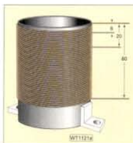
Fig. 3a & b: Coil winding details for the wavemeter project (see text).
