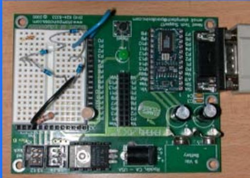
I programmed the BS2SX chip that is in this prototyping board. It determined if the pin that was connected to the RF bridge rectifier was TTL high. If the pin was high then an LED would be toggled from green to red. I used the following source code to do the trick.
