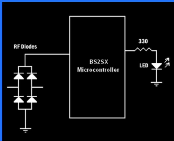
This is the simple unamplified true/false detector that senses the cell phone when the RF bridge rectifier sets the microcontroller input to high.
