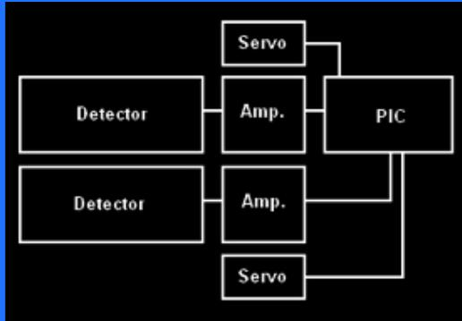
This is a simplified hook up diagram for the device. The A/D converter isn't shown.
