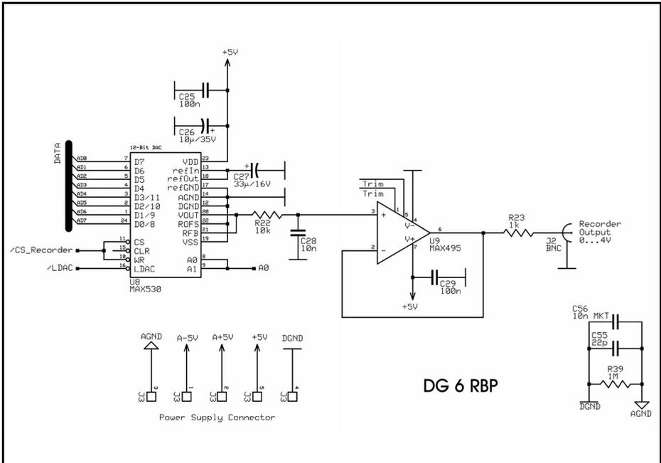
**Fig 3: Recorder output for the digital mW meter.**
