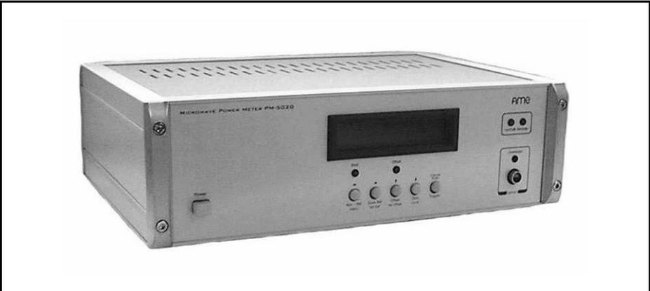
**Fig 4: Completed digital mW meter by DG6RBP.**
