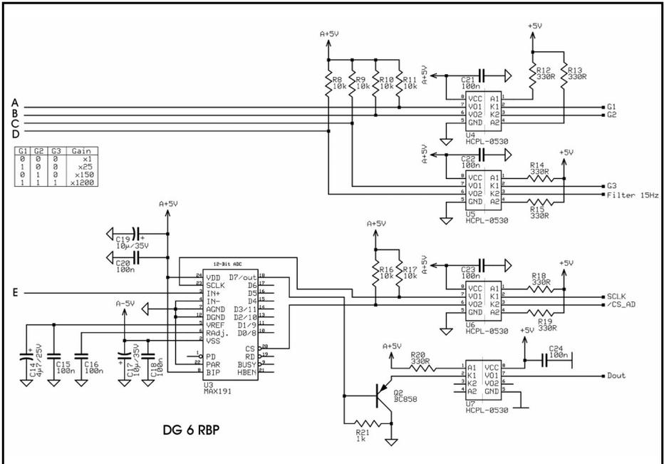
**Fig 2: A/D converter for the digital mW meter.**
