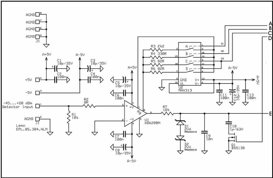
**Fig 1: Input amplifier for the digital mW meter.**
