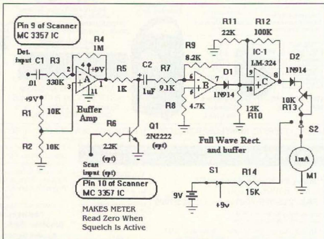
Figure 1. Schematic for the FM Packet Deviation Meter.
