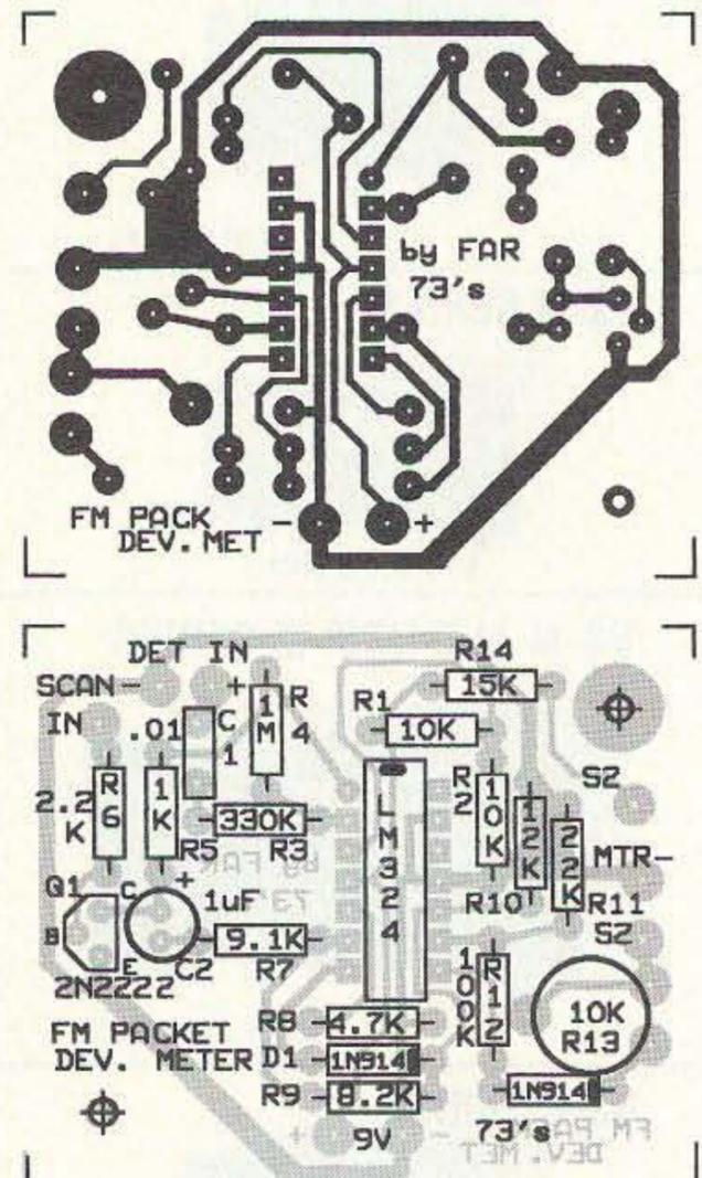
Figure 2. PC board pattern and parts placement diagram.
