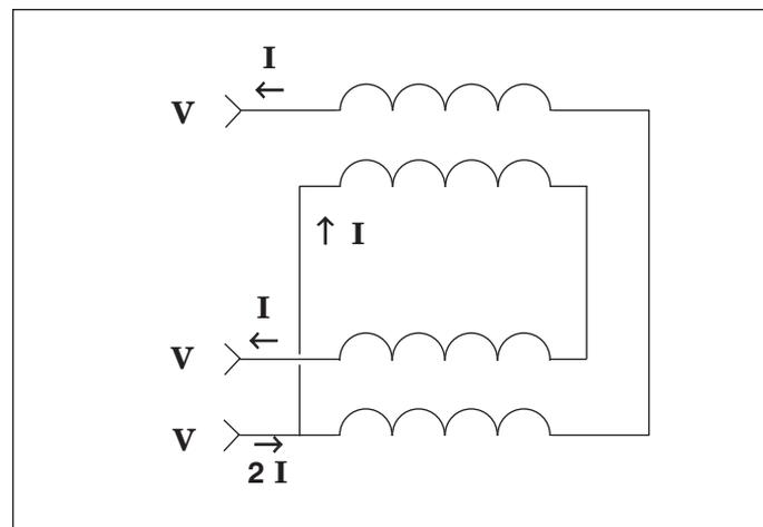
▲ Figure 3. Type II combiner/splitter circuit.
