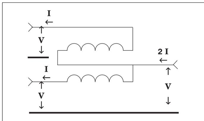
▲ Figure 2. Type I power combiner/splitter circuit.
