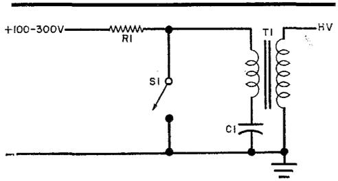
Fig. 3. When  $S1$  is closed,  $C1$  discharges through primary of transformer producing the high-voltage spike.
