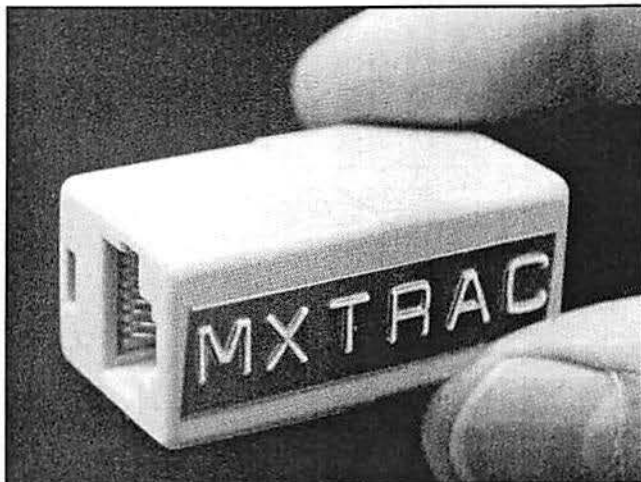
RJ-type modular connectors are used in the Maxtrac radios, so a double-ended female 8-pin RJ modular connector device was chosen to house the link. This forces compact wiring, and short leads are required in such configurations to reduce the possibility of stray RF pickup.
