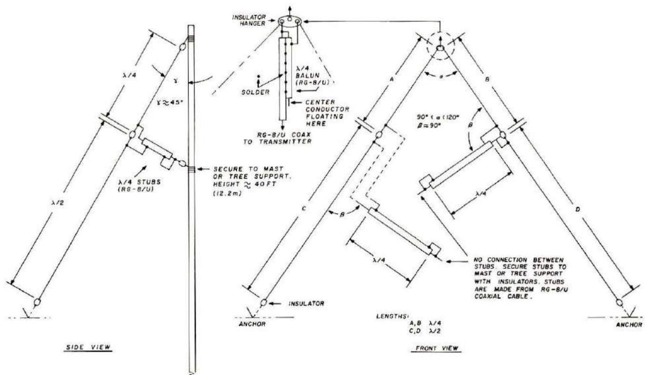
**Fig. 3.** The modified inverted-V antenna. Two half-wavelength elements are added, which are driven in phase. The angles shown are nominal. The coax cable is shown as RG-8/U, but RG-58/U will work for low-power transmitters. Good solder connections are important for trouble-free operation.
