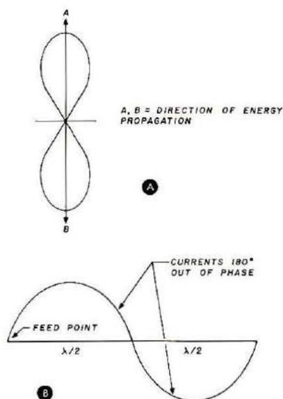
**Fig. 2.** Radiation pattern of an antenna with two half-wave elements driven in phase, **A**. The pattern is sharper than that of an ordinary dipole and gives increased signal strength in the directions shown. Sketch **B** shows the current distribution in two half-wavelength antenna elements connected directly together; that is, the system operates as a full-wavelength antenna.
