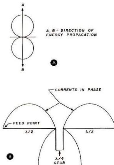
**Fig. 1.** Radiation pattern for a simple horizontal dipole antenna, **A**, and current distribution of two dipoles driven in phase, **B**.
