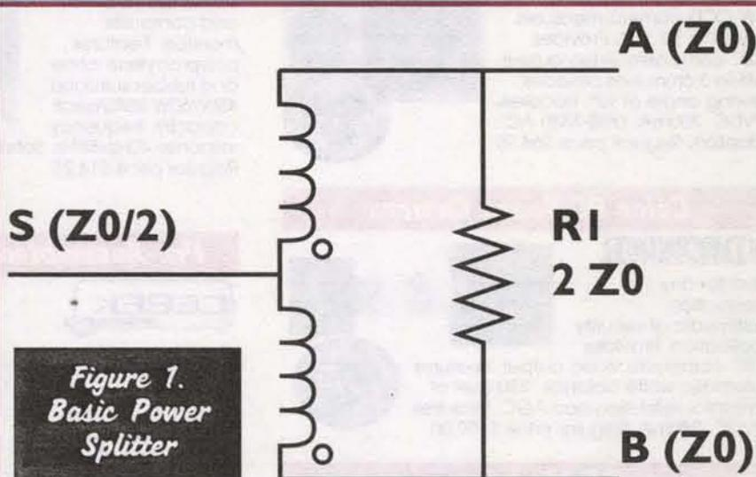
Figure 1. Basic Power Splitter
