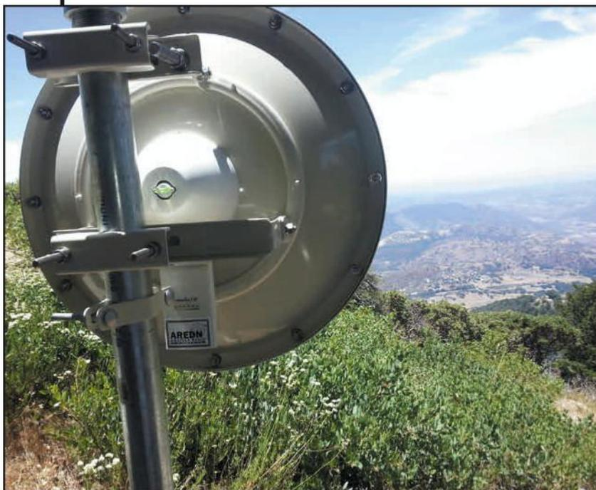
Figure 1. A Ubiquiti Rocket M3 serving as an AREDN™ node. On these frequencies, line of sight is important, so long-haul backbones tend to be at good sites. EmComm users could then deploy portable nodes to deliver “last mile” connectivity into an area, providing intranet connections between an EOC or other operational command center and its deployed resources. (Courtesy of AREDN)
