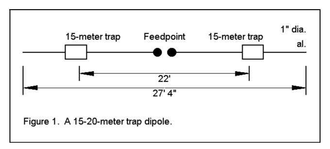
A trap consists of an inductance and a capacitance, normally resonated just at or below the lowest frequency of the higher antenna frequency range. The limiting factor in a trap is the resistive loss of the coil, since the losses in capacitors at HF are very small. A trap effectively consists of a series combination of resistance and inductive reactance in parallel with capacitive reactance. See Figure 2a.
