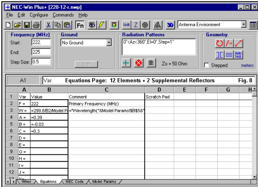
**Fig. 8** shows the very simple equations page, with 3 variables, A, B, and C. A is the element half length in meters (the default unit of .NEC-format conversion from EZNEC to NEC-Win). B is the distance along the Y-axis, where a value of zero would align the new reflectors with the old. C is the vertical separation of each reflector above and below the plane of the other elements.
