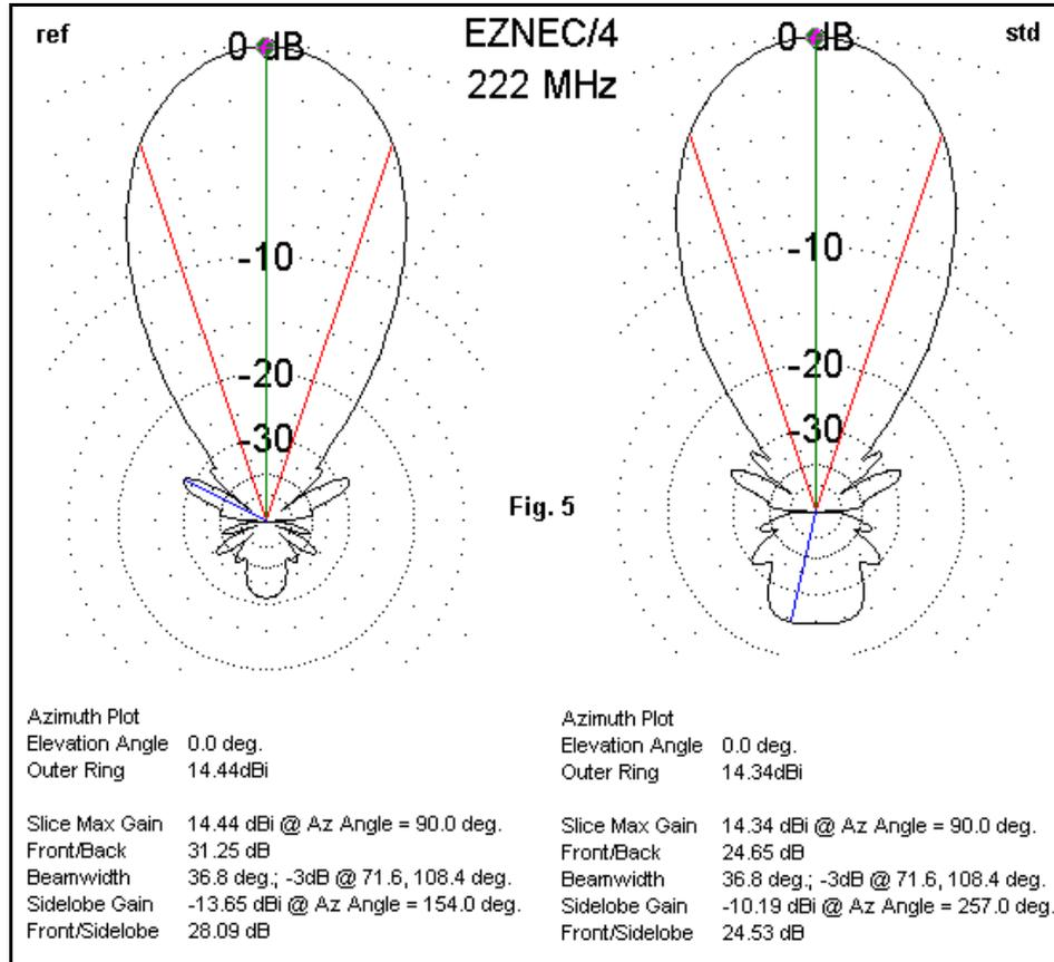
**Fig. 5** shows the corresponding patterns at 222 MHz. Most notable is the shrinkage of the main rear lobe, but without significant effect on the rear side lobes. The strongest rear side lobes remain virtually as strong in both patterns, although the main lobe shrinkage makes those lobes more vivid for the ref model. In fact, a new set of rear side lobes, swallowed by the main lobe in std, becomes evident in ref.
