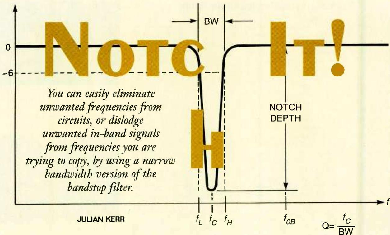
Anyone who builds or experiments with electronics circuits has at one time or another been faced with the problem of removing unwanted frequencies from the signal of interest. In most cases, a simple low-pass, high-pass, bandpass, or band-reject filter will suffice. Such filters are great for blocking entire bands of frequencies, but what do you do when the offending frequency is within the band of interest?
