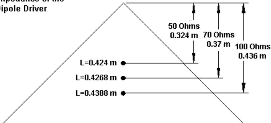
Because the mutual coupling between the reflector and the driver decreases with additional distance between the driver and the reflector surfaces, we find that the dipoles grow longer as they move away from the apex. More significantly, the lessening of mutual coupling also increases the SWR bandwidth, as shown in **Fig. 23**. For each curve, the SWR reference is equal to the resonant impedance of the driver.
