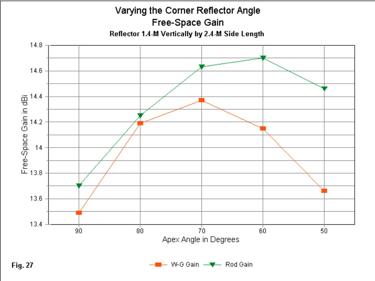
Wire-grid gain peaks at an angle of about 70 degrees, but the rod-reflector requires a narrower angle for peak gain, something just over 60 degrees, if we read the peak values correctly. The following table provides a more detailed look at comparative numbers as we reduce the angles for both types of reflector.
