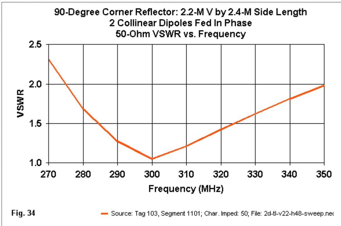
The 50-Ohm SWR curve appears in **Fig. 34**. The acceptable (2:1) SWR level exists from 275 to 350 MHz, a 75-MHz passband. Expressed in other terms, we have a 25% passband with respect to the 2:1 50-Ohm SWR standard when referenced to the design frequency. Not only is the feedpoint impedance well behaved across this range, but as well, the E-plane and H-plane patterns are paradigm examples of what a corner reflector can achieve. **Fig. 35** provides a pair of samples from the design frequency.
