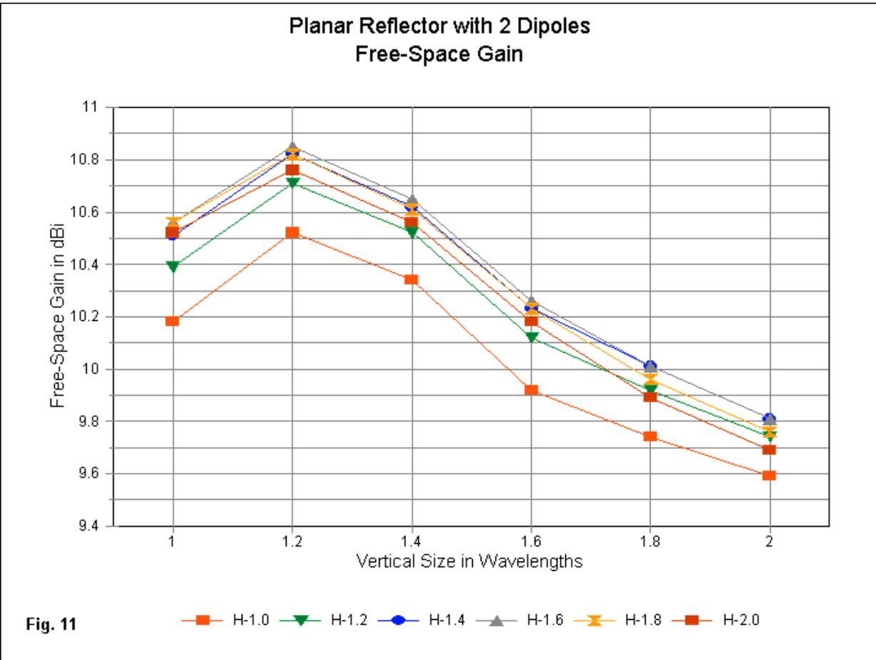
The detailed performance values for a planar reflector array using 2 dipoles fed in phase appear in the next lines. The impedance value shown is for each dipole prior to the addition of the phase lines.
