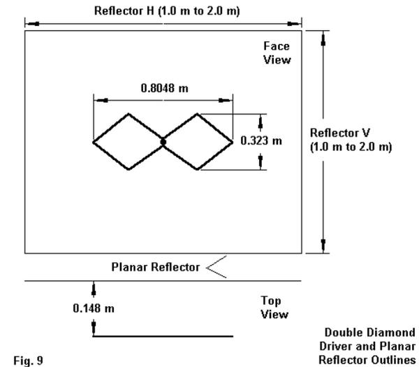
Each driver requires a set of dimensions that, in isolation, maximizes bi-directional gain. Hence, most of these vertically polarized arrays are somewhat squat. That is to say, they are extended horizontally to approach a spacing of  $\frac{1}{2}$ -wavelength between the high-current regions of the elements, thus shortening the vertical elements from a nominal  $\frac{1}{4}$  wavelength. The spacing from the planar reflector for each driver derives from the inherent resonant feedpoint of
