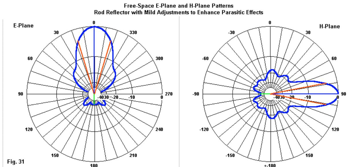
The patterns clearly show the hybrid nature of the modified reflector structures. The beamwidths are typical of corner arrays, but the emergent sidelobes are more typical of parasitic arrays, such as Yagis. The following table compares the performance reports of a standard 70-degree corner reflector and one of the enhanced parasitic designs.
