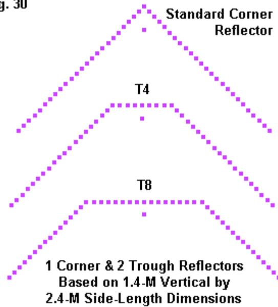
The following table records the results of the survey. The model identification records the amount cut off from the apex, where T2, for example, means that 0.2 wavelength has been removed and replaced by a flat surface. The largest troughs result in a split forward H-plane lobe that has a central null that is greater than 3 dB.
