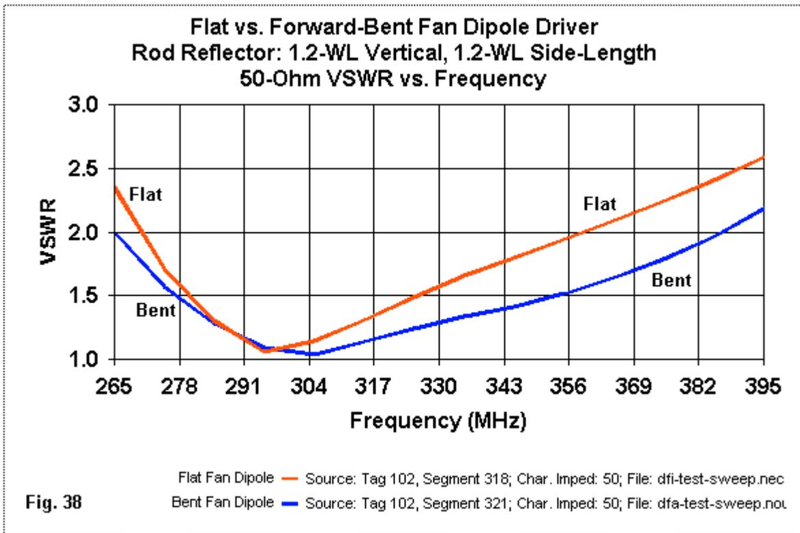
The passband increases further if we re-design the bent fan dipole for a higher impedance. Preliminary models have come close to the original 300-400-Ohm impedance and have also shown considerable improvement over the already wide 50-Ohm passband. However, present models are not yet reliable enough to be more than suggestive in this regard.
