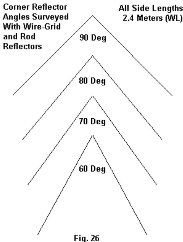
To see what we might gain, if anything, from a narrower corner angle, I surveyed both wire-grid and rod corner reflectors using 1.4-wavelength vertical reflectors having a side length of 2.4 wavelengths. **Fig. 27** shows the results in terms of the free-space forward gain.
