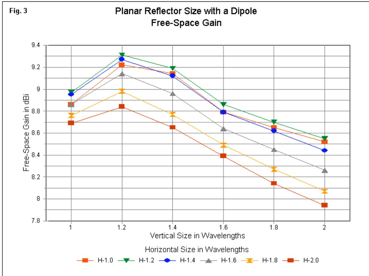
At maximum gain with a 1.2-wavelength by 1.2-wavelength reflector, I obtained the following performance reports. The front-to-back value is for 180 degrees. E-BW and H-BW are the -3-dB beamwidths for the E- and H-planes, respectively.
