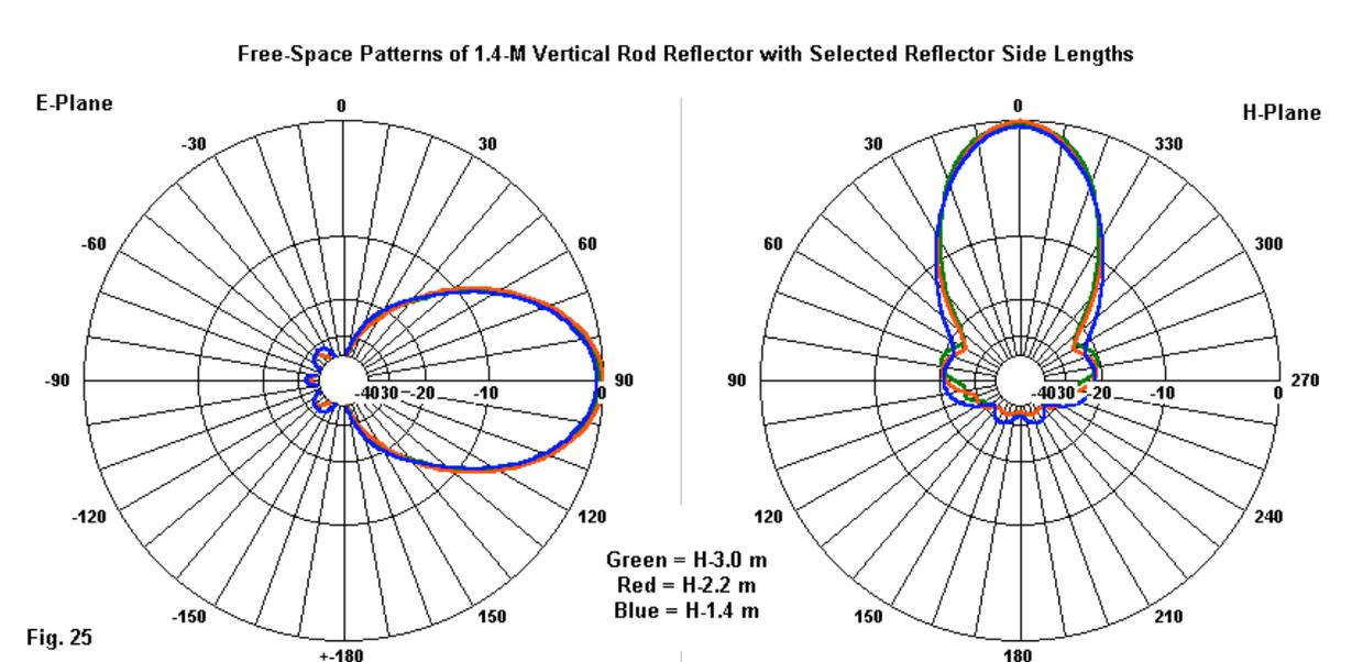
Relative to wire-grid patterns for maximum gain, the patterns for a maximum gain rod reflector do not exhibit any significant anomalies. **Fig. 25** overlays patterns for a 1.4-wavelength reflector with side lengths of 1.4, 2.2, and 3.0 wavelengths. At most, we obtain
