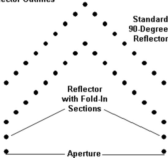
The test series has used rod reflectors 1.4 wavelength high. Since the maximum gain of such a reflector occurs with a 60-degree angle, I added a single rod to the side length in standard fashion and then did a fold-in instead. The following table shows the results.
