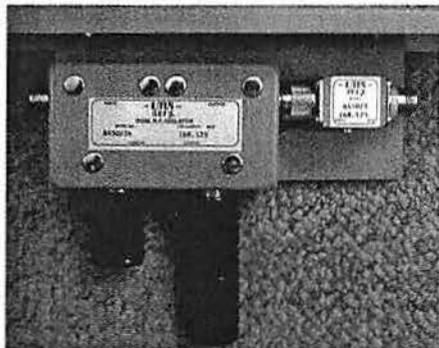
The dual isolator has a larger dummy load connected to the side of the isolator that is close to the antenna line.
