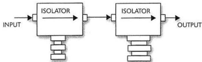
Figure 4. Two isolators can be connected in cascade as shown here to increase the amount of isolation. Make certain that the larger dummy load is located on the isolator nearest the output or load side.
