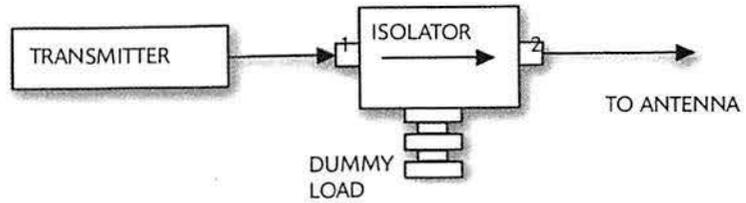
Figure 3. The isolator is connected directly to the output of the transmitter with the #1 port connected to the transmitter and the #2 port connected to the antenna. Any reflected power is dumped into the dummy load.
