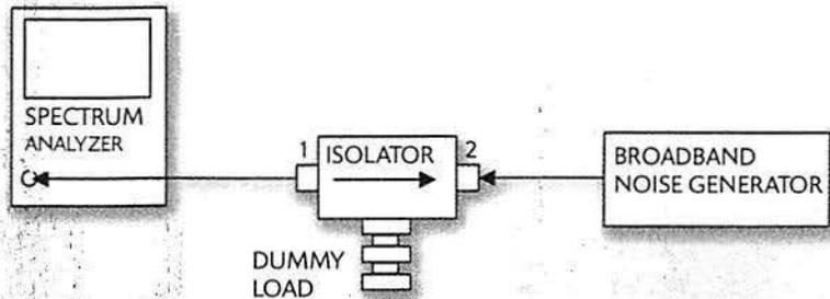
Figure 2. A broadband noise generator is used to check the frequency response of this isolator in the reverse direction.
