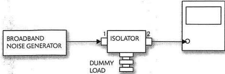
Figure 1. A broadband noise generator is used to check the frequency response of this isolator in the forward direction.
