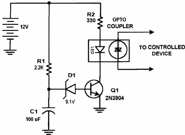
THIS CIRCUIT PRODUCES A DELAY IN TURNING ON THE OPTOCOUPLER USING COMPONENTS R1, C1, D1, AND Q1
