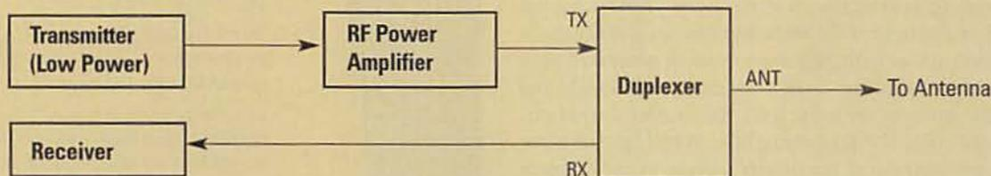
This is a typical repeater arrangement. The RF amplifier may not like the load presented by the input to the duplexer. The line length between the duplexer and the RF amplifier output may be changed to improve the load impedance to the RF power amplifier.
