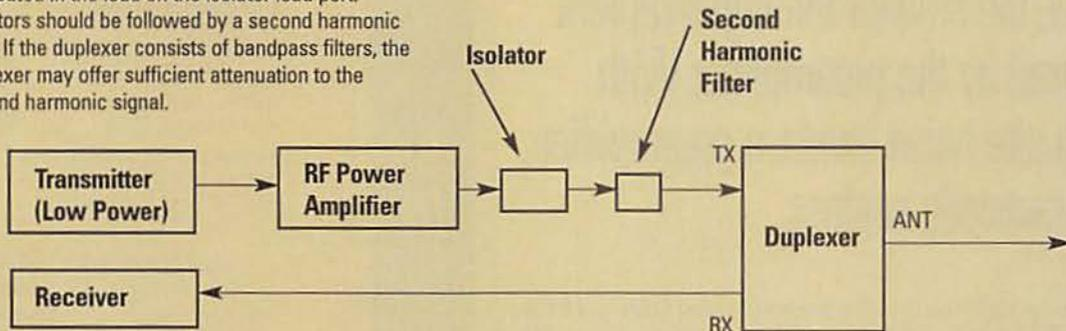
narrow band of frequencies over which the amplifier must operate. In the case of a transceiver, the RF amplifier must have a bypass that allows the receive signal to pass through the amplifier in the reverse direction with little attenuation.
