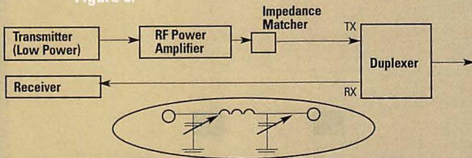
An impedance matcher such as the pi-network shown in the inset can be used to provide a proper match to the RF power amplifier. Such impedance matchers are designed to mount right on the output connector of the RF amplifier. Tuning adjustments are accessible through small holes usually covered by caps to keep dust and other foreign matter out of the device.
