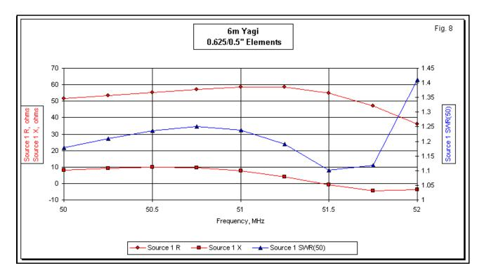
To scale the designs down to 50.5 or to 50.1 MHz, use the same factors applied to the uniform-diameter elements (1.01 and 1.018, respectively). Apply these only to the tip sections, leaving the inner sections at 24" for a half length (or 48" for a full length). In fact, a 1%-2% change in the length of the inner sections will make no noticeable difference to beam performance. Remember to scale the element spacing as well as the element lengths.
