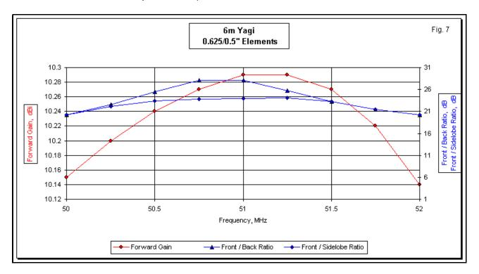
To obtain the very good OWA-type performance curves for gain and front-to-back ratio, the SWR curves suffer slightly. The values for 50 and 51 MHz shows a decrease in 50-Ohm SWR as we increase the element diameters. However, the value for 52 MHz show increases with larger elements. However, the highest value modeled is comparable to the highest value modeled for the uniform-diameter elements. See **Fig. 8**.
