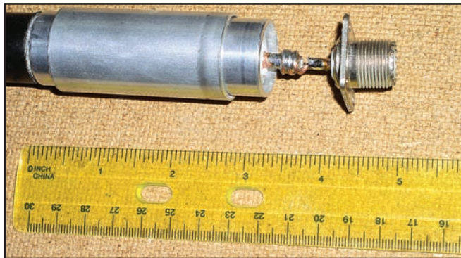
Figure 3 — Detailed view of center conductor connection method.
