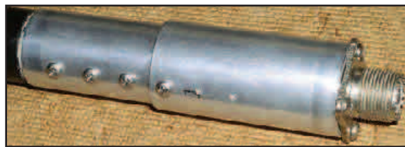
Figure 4 — The outer tubing sections secured with shortened sheet metal screws.
