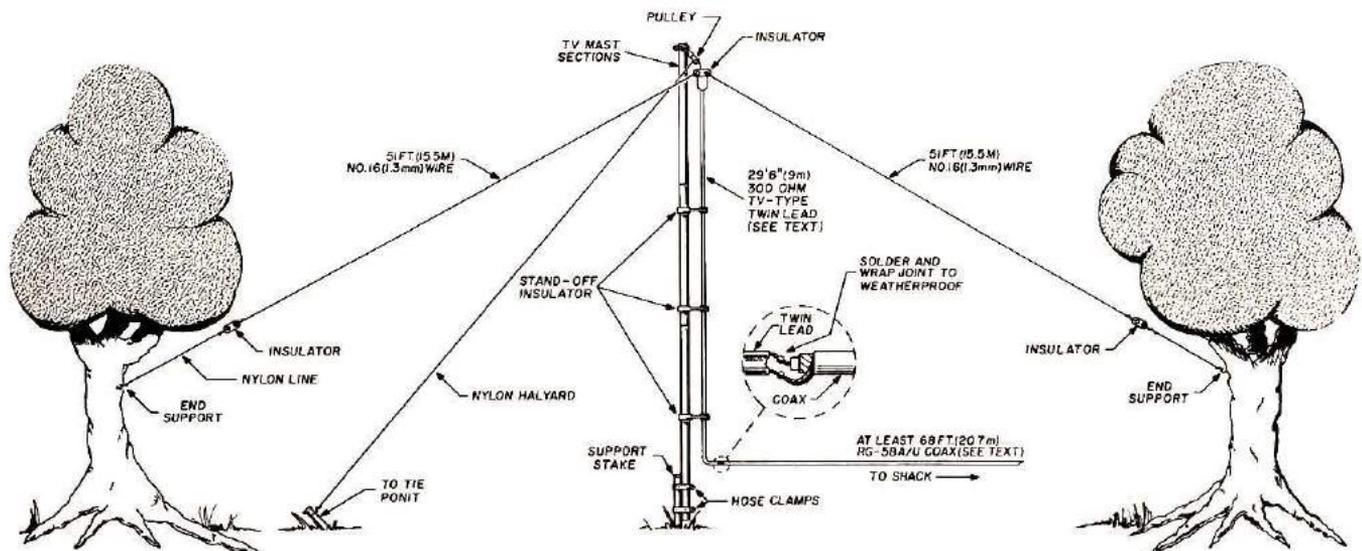
In this instance, the G5RV antenna is shown in an inverted-vee configuration. A nylon halyard raises the center of the antenna to the top of a mast made from TV mast sections. Stand-off insulators keep the feedline from flapping in the wind. The antenna "legs" serve as guy wires, while the halyard acts as additional support.
