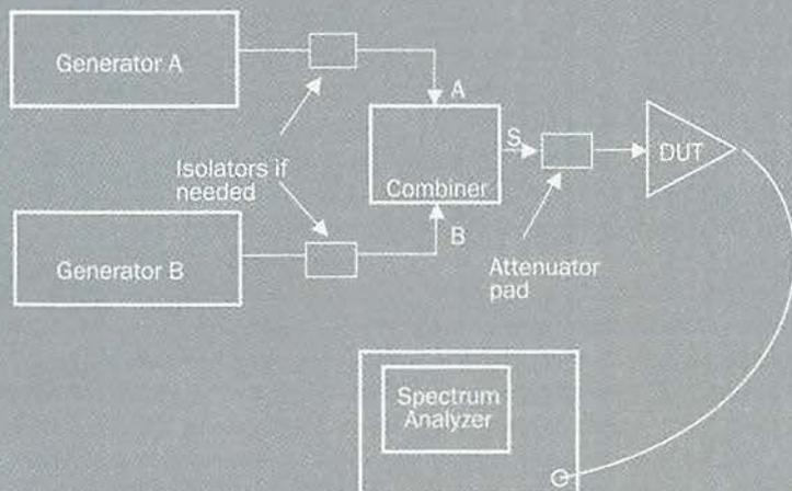
This test setup is used to check the intermodulation distortion (IMD) performance of the DUT (device under test), a small-signal RF amplifier. See text for full discussion.
