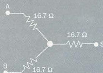
A resistive combiner such as this could be used to combine the signals from two signal generators. However, not enough isolation would be provided between the signal generators. Additional means of isolation would be required.
