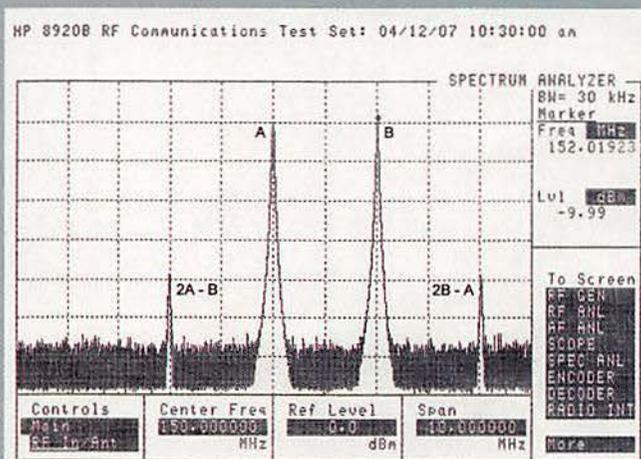
This spectrum analyzer display shows the two CW tones (A and B) and the resultant third-order I-M products (2A-B and 2B-A). See text for details.
