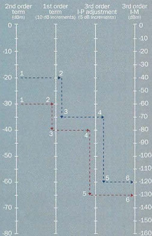
Figure 5: This nomogram can be used to determine the level of the third-order intermodulation product produced in the output of an amplifier, given the output level of the fundamental tones, A and B, and the third-order intercept point of the amplifier.
