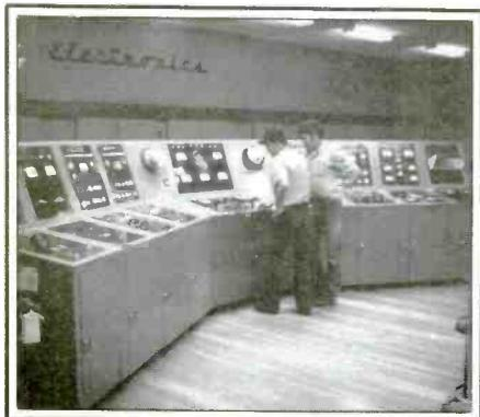
The only station in the world using an AN/FRT-31 transmitter is NAVCOMMU Cutler. Here's how the massive control panel looks.
