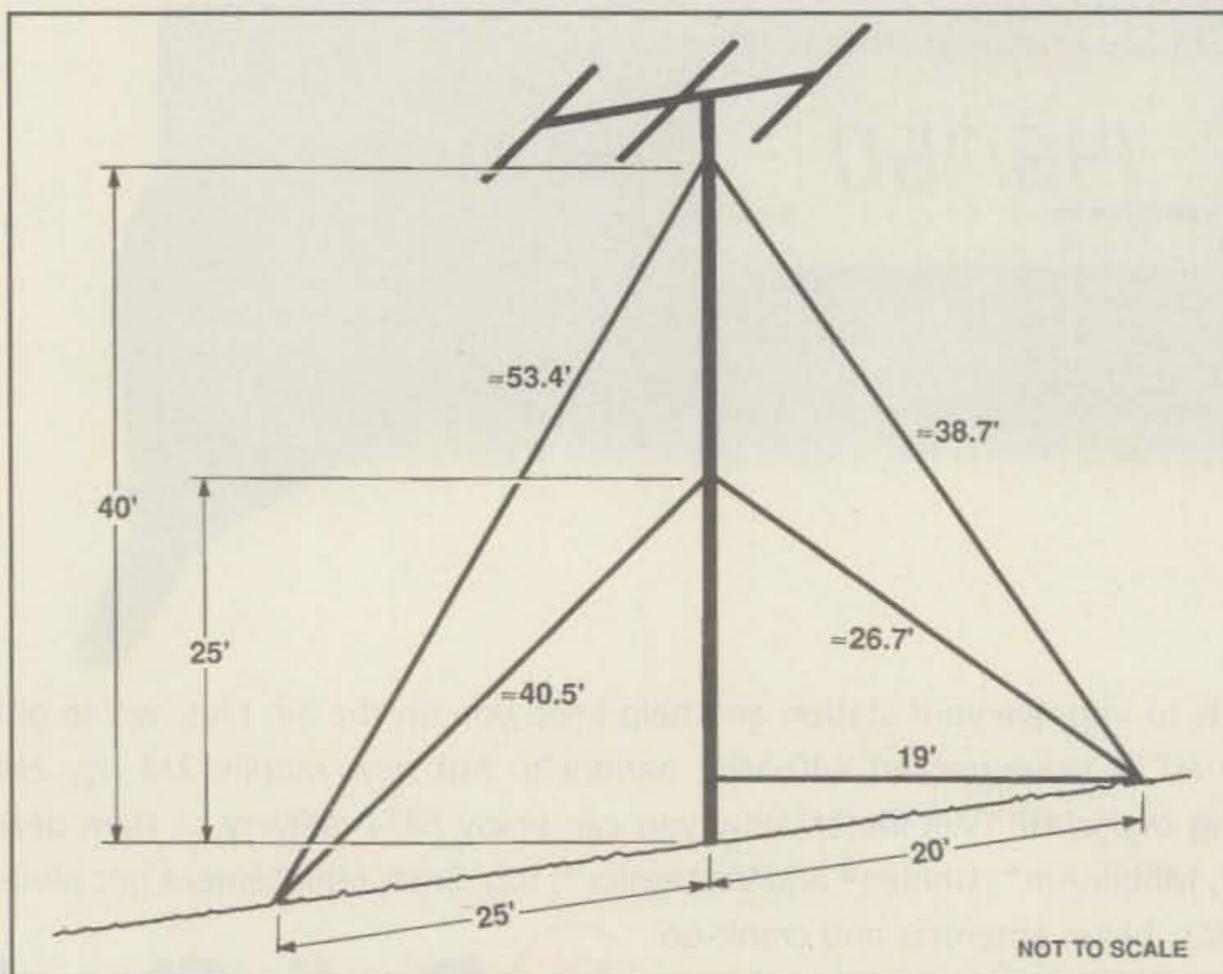
Fig. 3—If you live on an incline, there is an alternative to renting a bulldozer to flatten it out.
