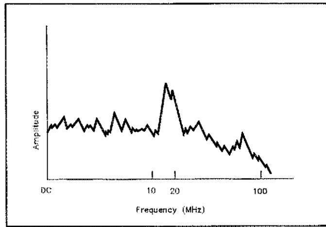
Fig 2—Spark-generated interference may not generally decrease in strength with rising frequency when power lines associated with the noise source resonate and peak the noise at one or more frequencies.
