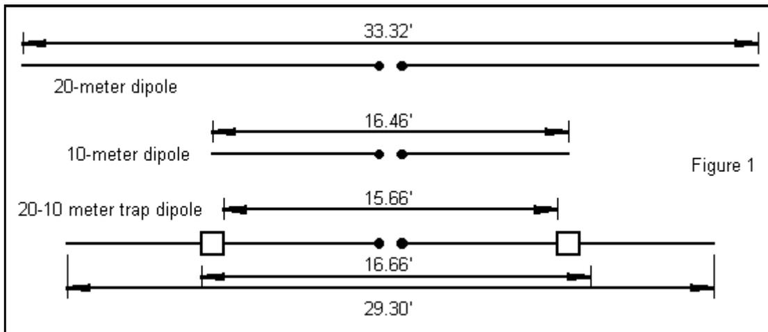
The dimensions of the model in Figure 1 should draw some attention. Compared to a 10 meter dipole with a length of 16.46, the 10 meter inner wire's length of only 16.66' indicates that the load is mostly within the standard 10 meter length. The segments of the antenna are roughly 0.5' each, and the loaded segment is on each end. A load is distributed throughout the segment, although
