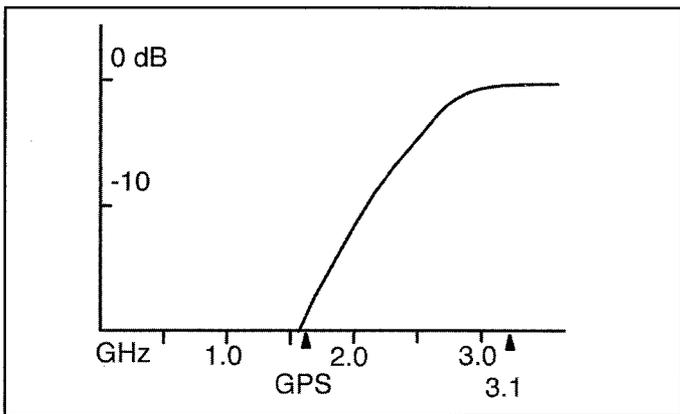
Figure 3. Gaussian response filter protecting GPS.
