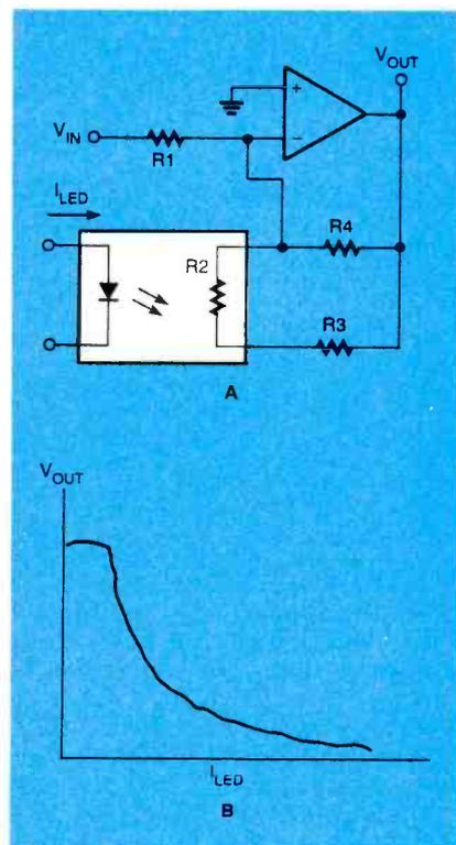
Fig. 6. Analog optoisolator/couplers can also be used as gain controls as shown in A. The gain of the op-amp is affected by changes in the resistance of the photocell caused by light radiation. The  $V_{OUT}$  vs.  $I_{LED}$  characteristics of this gain-control circuit is shown in B.
