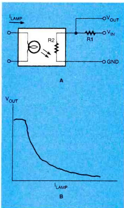
Fig. 4. The photocell type analog optoisolator/coupler is well suited to attenuation applications. In A, the unit's photocell output serves as a shunt resistor. The  $V_{OUT}$  vs.  $I_{LAMP}$  characteristics of this circuit is shown in B.
