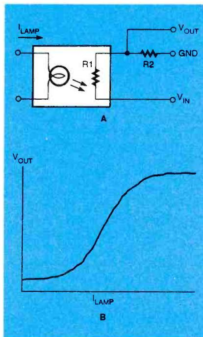
Fig. 5. Here is another optoisolator/coupler attenuation circuit. In A, the photocell is connected as the series resistor. The  $V_{OUT}$  vs.  $I_{LAMP}$  characteristics of this circuit is shown in B.
