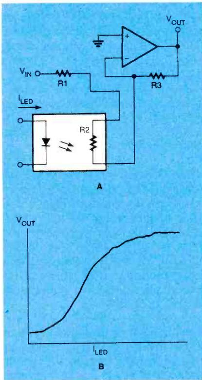
Fig. 7. In the gain-control circuit shown in A, the gain of the op-amp is affected by varying the magnitude of the input signal. The  $V_{OUT}$  vs.  $I_{LED}$  characteristics of the gain control circuit is shown in B.
