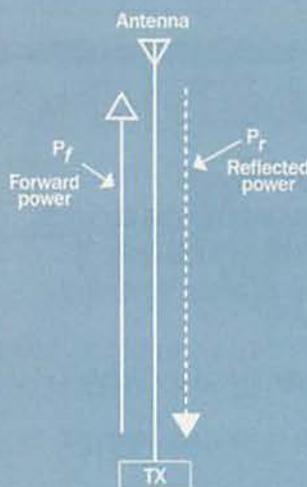
In Figure 1, a transmitter is connected to an antenna through a 100-foot length of transmission line. Let's suppose in this instance that the transmission line is loss-less (though no such circumstance exists in the real world.) Further suppose that the antenna is not properly matched to the 50 ohm system and that 25% of the RF power is reflected back down the line from the antenna toward the transmitter. With the in-line directional
