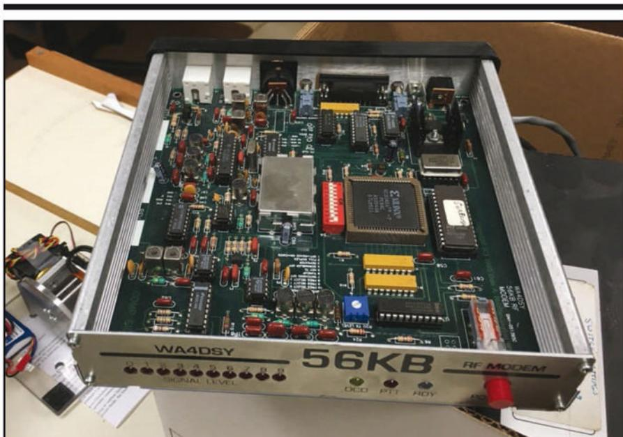
Photo B. A later-version WA4DSY 56k-Baud Modem. At upper left, the white cubes are the backs of the BNC RF in and out connectors. The FPGA is the large Xilinx chip center right, and to the right of that is the EPROM containing the FPGA programming data, waveform tables, modem state machine, TX/RX frequency data and the "secret" remote control codes to optionally allow for a remote PC reset.
