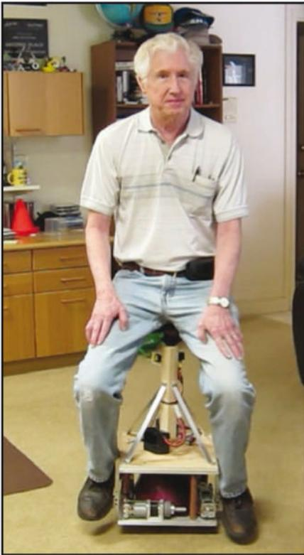
Photo C. WA4DSY is demonstrating the output of one of his design sessions for me: iRoll, a self-balancing stool that uses a bowling ball as its wheel. It was absolutely frightening to watch him get on this thing, but it was as stable as a rock. I declined to give it a try, citing some imaginary fear of death and lack of faith in technology.
