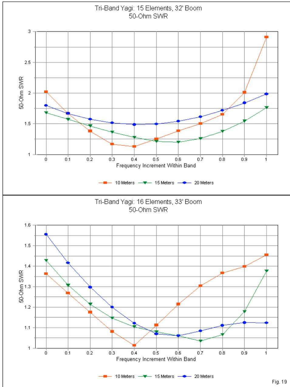
Direct coupling of the drivers does ease the problem of obtaining a low SWR across each of the HF bands covered by the antenna. The lower part of **Fig. 19** shows excellent curves when measured by tri-band standards. (Remember that we cannot expect of a tri-band Yagi the same smooth performance curves that we obtained from the short-boom 6-, 7-, and 8-element monoband Yagis.)
