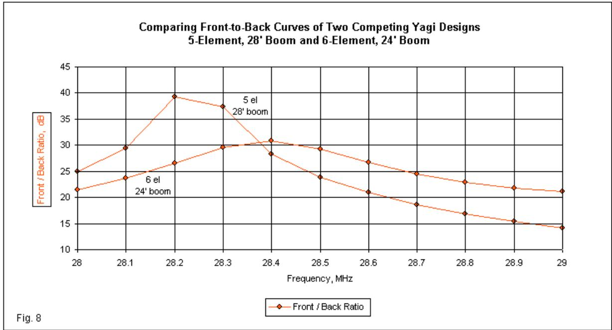
We can make the 5-element Yagi stand out by citing the peak front-to-back ratio: about 39 dB. However, the 180° front-to-back ratio varies across the band from the peak value down to 14 dB. In contrast, the 6-element beam shows only a 9-dB variation in front-to-back ratio, varying from a low of 21 dB to a high of over 30 dB. In this comparison, the average front-to-back ratio values would tell us very little, since they are within about 0.8 dB of each other.
