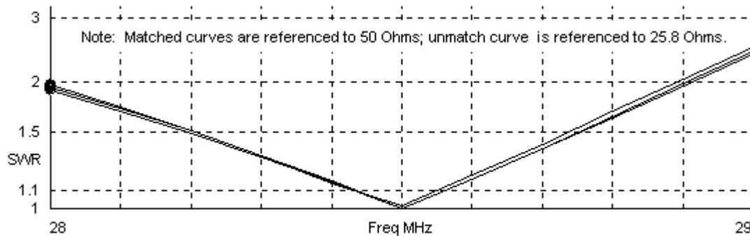
Overlaid SWR Curves of the 3-Element Long-Boom Yagi with No Match,
