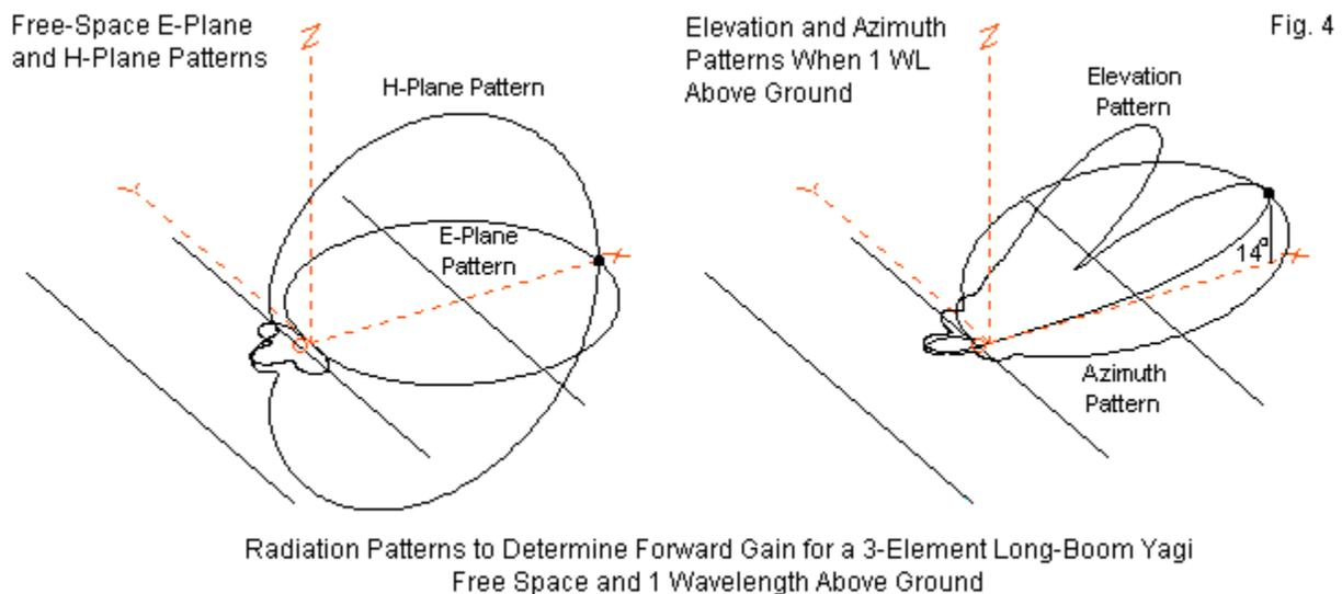
On the left, we find a 3-element Yagi (our long-boom sample) and the E-plane and H-plane patterns associate with the free-space environment. As noted earlier, the E-plane pattern aligns with the plane formed by the 3 elements. The H-plane pattern is at right angles to the E-plane pattern, when both patterns use the same heading for maximum gain. Note that the patterns meet at the maximum gain point and again at the point that is 180° from the maximum gain heading.
