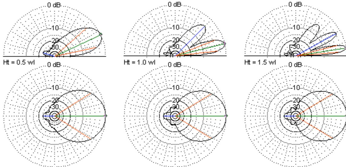
3-Element Long-Boom Yagi Elevation and Azimuth Patterns at 3 Heights Above Ground
