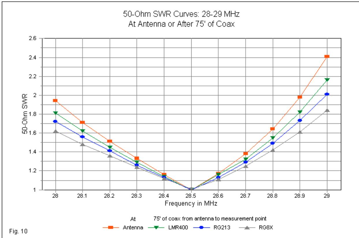
The results of the test appear in **Fig. 10**. The steepest SWR curve belongs to the antenna terminals with no cable. Since every cable has some loss, all cable curves are broader than the cable-less curve. The curves become broader as the cable loss increases. The only curve that manages an SWR under 2:1 across the entire passband is RG-8X, the lossiest of the collection. (Very lossy RG-58 would show an even broader SWR curve. As cable loss increases, less power reaches the antenna.)
