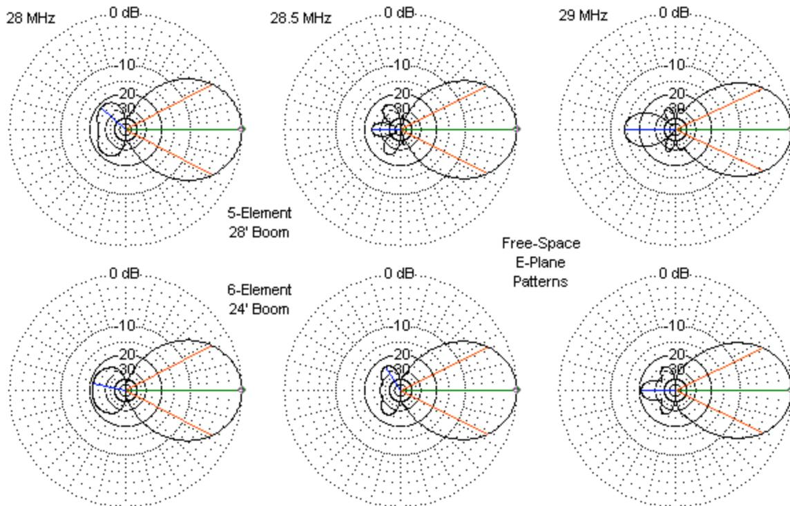
Comparing Azimuth Patterns of Two Competing Yagi Designs
