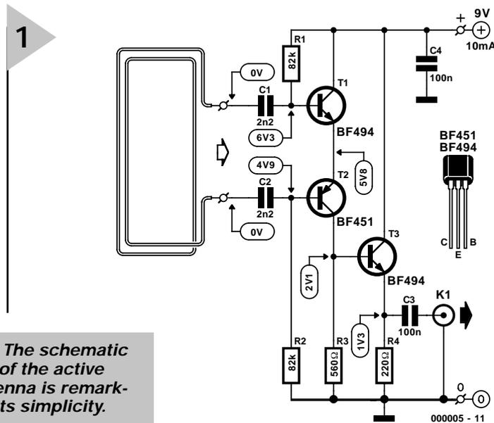
**Figure 1.** The schematic diagram of the active loop antenna is remarkable for its simplicity.
