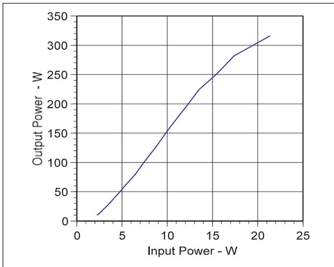
■ **Figure 6. Output power vs. input power with the amplifier set up for 300-watt CW operation.**
