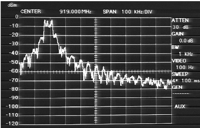
■ **Figure 7a. Wideband measurement of sidebands from the simple transmitter: BFSK.**
