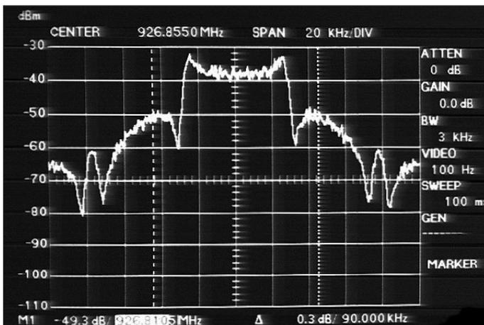
■ Figure 3. Spectrum of the BFSK test signal with markers showing the bandwidth predicted by Carson's Rule.
