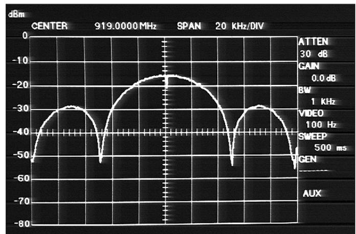
■ Figure 4. Spectrum of the BPSK test signal showing the width of the main lobe is 100 kHz, twice the data rate.
