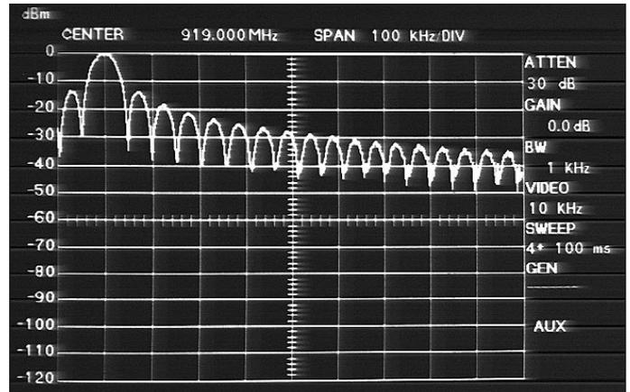
■ **Figure 7b. Wideband measurement of sidebands from the simple transmitter: BPSK.**
