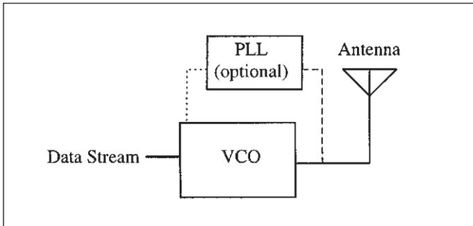
■ Figure 2a. Simple BFSK transmitter model.
