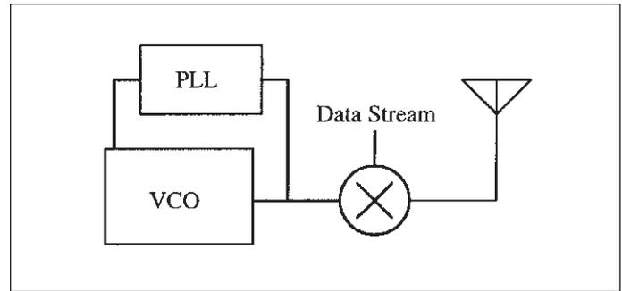
■ Figure 2b. Simple BPSK transmitter model.
