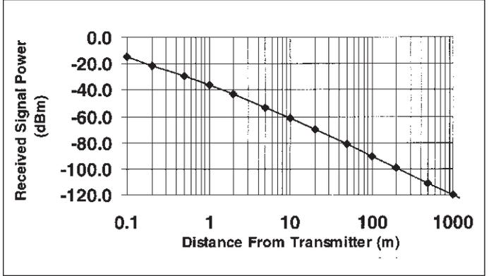
■ Figure 5. Received signal power vs. distance from the transmitter for the test scenario.
