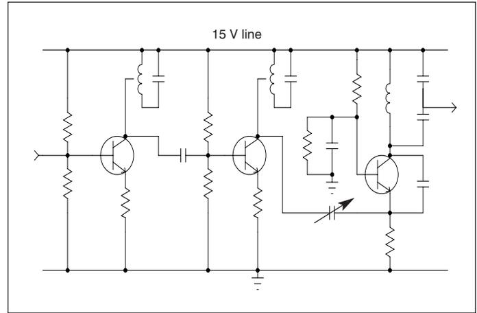
■ Figure 3. The transmitter IF filter.
