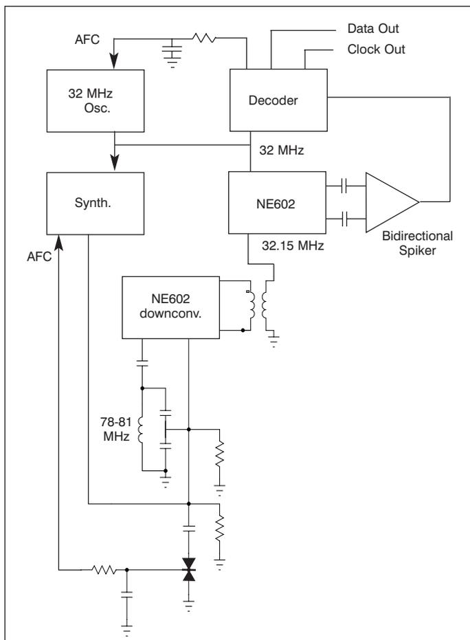
■ **Figure 7. Receiver IF and VPSK detector.**
