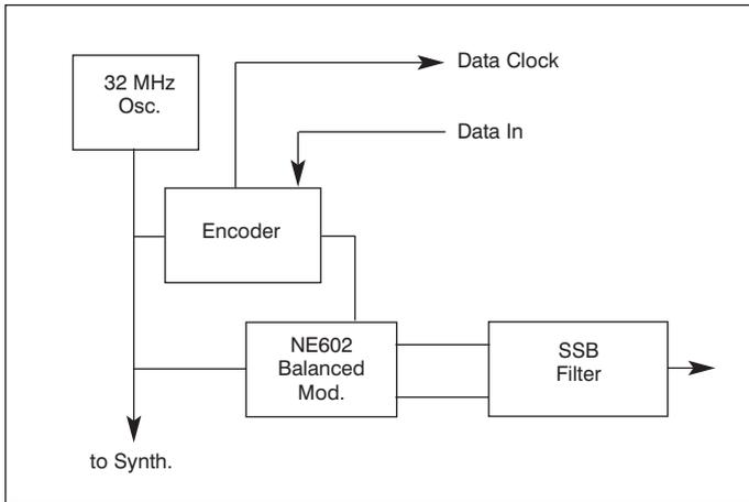
■ Figure 2. The data encoder and modulator.
