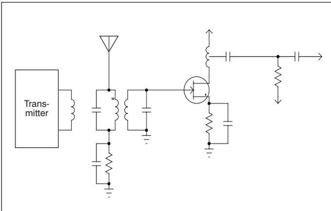
■ **Figure 6. Receiver input circuit.**
