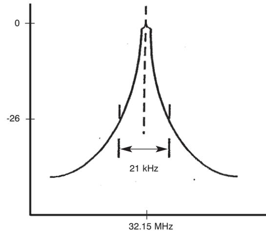
■ Figure 4. The spectrum for 320 Kb/s digital modulation using VPSK.
