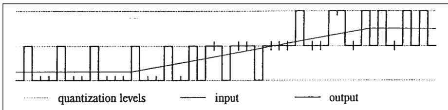
■ Figure 5. Generating “smooth” analog signals by high speed digital approximation.
