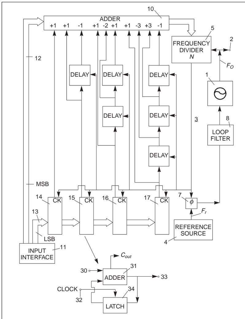
■ Figure 4. Diagram of the Marconi all-digital fractional chip from [8].
