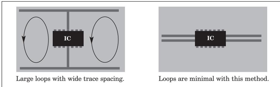
■ **Figure 3. Keep power conductors from creating large loops.**
