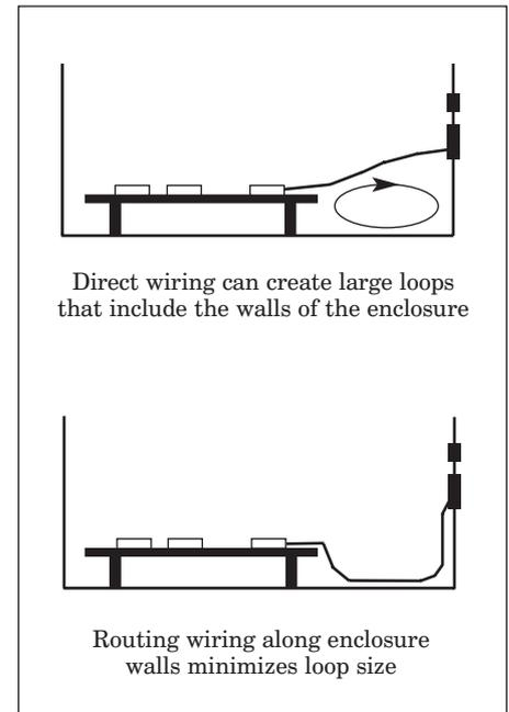
■ **Figure 4. Loop size can be controlled by routing internal lines.**
