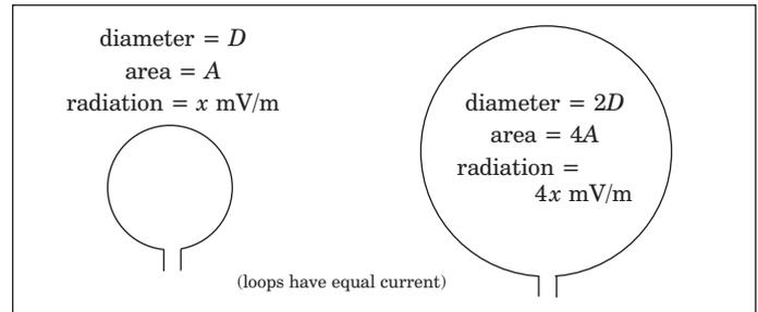
■ Figure 1. Radiation from loops is proportional to loop size.
