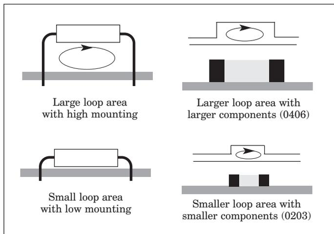
■ Figure 2. Component mounting affects loop size.
