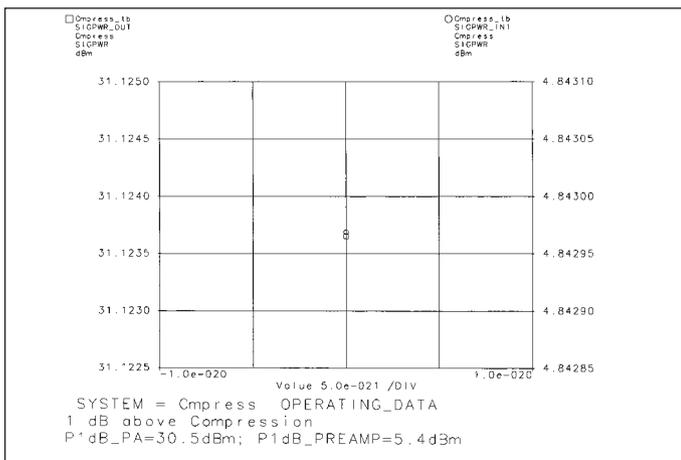
▲ Figure 7. Power amplifier output, 1 dB above  $P_{1dB}$ .
