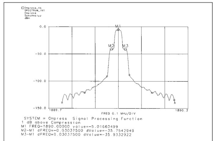
▲ Figure 8. Input signal spectrum, 1 dB above  $P_{1dB}$ .
