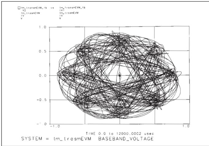
▲ **Figure 1. Encoded I versus Q constellation diagram.**
