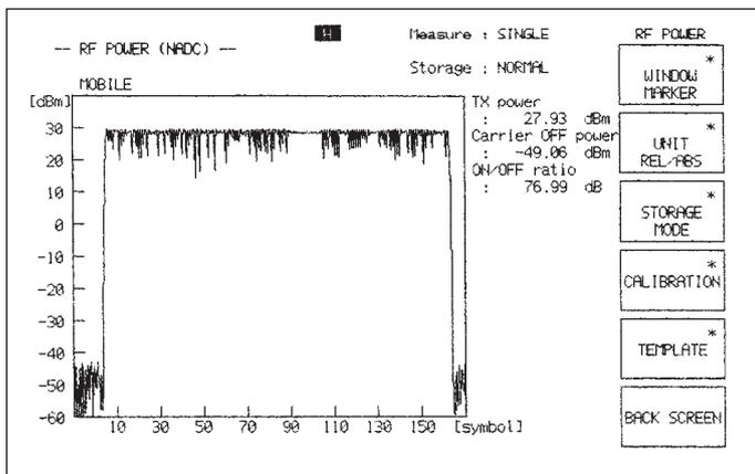
▲ Figure 15. TDMA power measurement of the amplifier.
