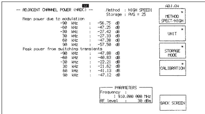
▲ Figure 14. ACP measurement results for the test amplifier.
