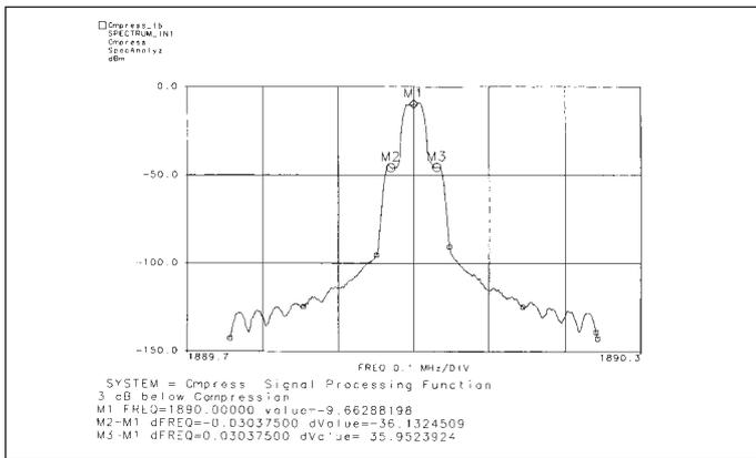
▲ Figure 11. Input signal spectrum, 1 dB below  $P_{1dB}$ .
