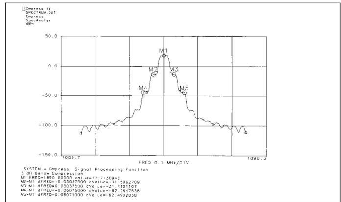
▲ Figure 12. Output signal spectrum at 1 dB below  $P_{1dB}$ .
