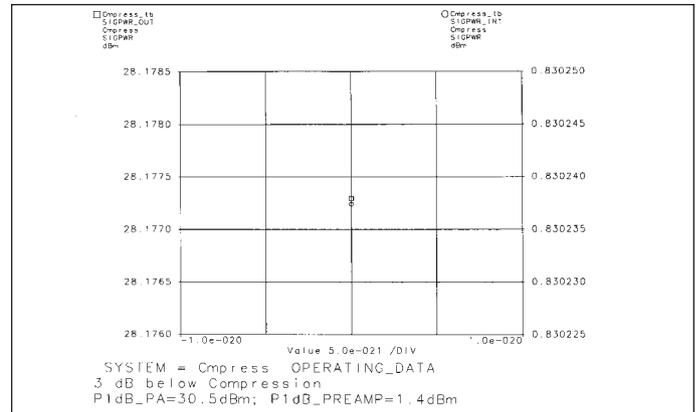
▲ Figure 10. Power amplifier output, 1 dB below  $P_{1dB}$ .
