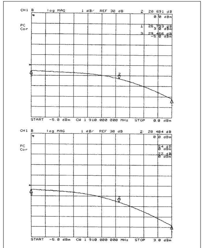
▲ Figure 13. CW power measurements using the RF2513 power amplifier, to determine  $P_{1dB}$ .
