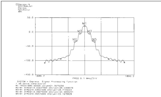
▲ Figure 9. Output signal spectrum at 1 dB above  $P_{1dB}$ .
