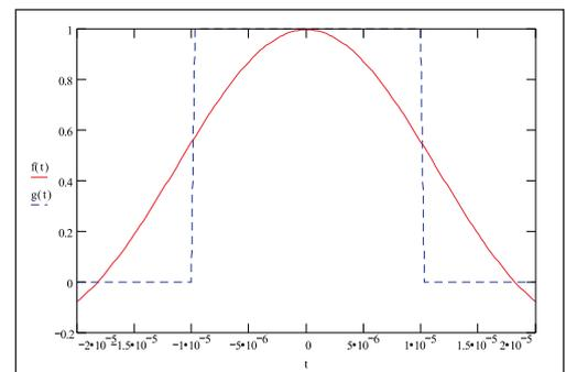
shaping application, the input signal does not have a constant amplitude any longer. It becomes an amplitude-modulated signal. The appearance of the amplitude modulation explains the spectrum spread to the adjacent channels. To understand the degree of the spread we must look at the properties of Gaussian-type pulses.
