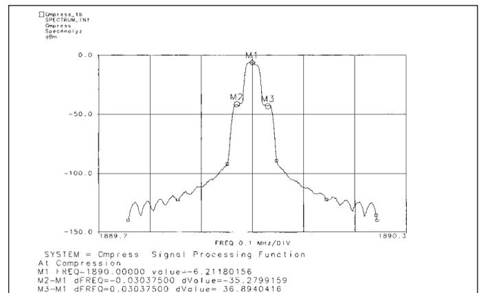
▲ Figure 5. Spectrum of the input signal.
