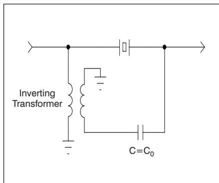
■ Figure 3. Alternate scheme for “inverted capacitance” cancellation.
