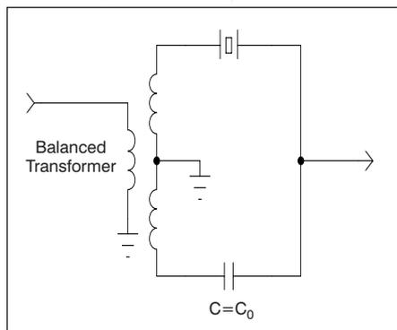
■ Figure 2. Balanced transformer network with “inverted capacitance.”
