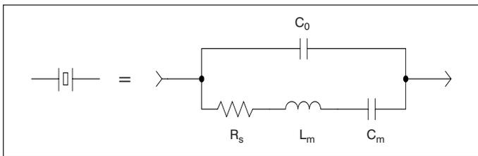
■ Figure 1. Equivalent circuit of a quartz crystal.
