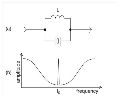
■ Figure 4. (a) Parallel resonant circuit and (b) its frequency response.
