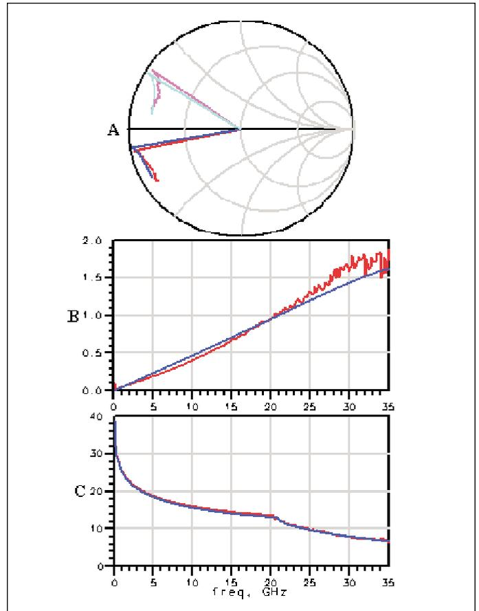
▲ Figure 5. (A) Reflection coefficients, red = input for data, blue = input for model, pink = output for data, light blue = output for model. (B) Stability factor,  $K$ , red = data, blue = model. (C) Max available gain, red = data, blue = model.
