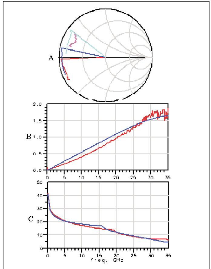
▲ **Figure 3. (A) Reflection coefficients, red = input for data, blue = input for model, pink = output for data, light blue = output for model. (B) Stability factor,  $K$ , red = data, blue = model. (C) Max available gain, red = data, blue = model.**
