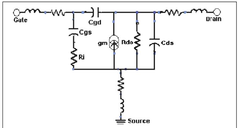
▲ Figure 1. Small-signal transistor equivalent circuit model.
