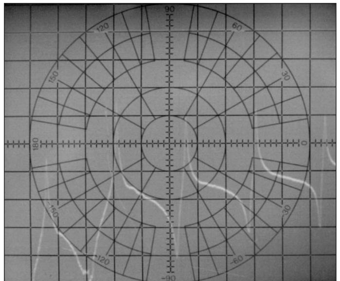
■ Figure 3. Transmission amplitude response of the vertically mounted solenoid in Figure 2. The sweep range is 500 kHz to 1300 MHz (approximately 108 MHz/DIV).
