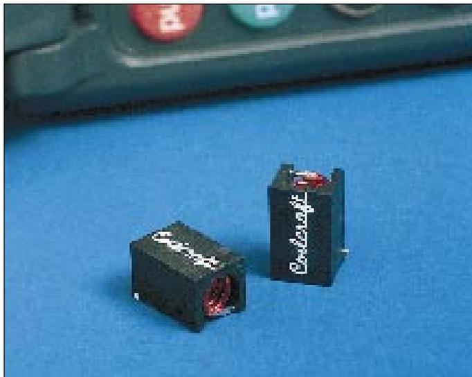
■ **Figure 12. Coilcraft 132 surface mount series of solenoid inductors.**
