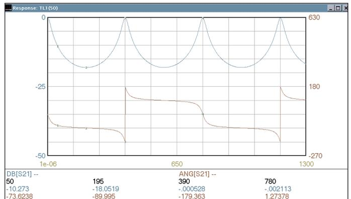
■ **Figure 7. Transmission amplitude and phase response of the simple proposed transmission line model for inductor. Transmission line impedance and length are adjusted to match the measured response.**
