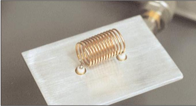
■ **Figure 4. Horizontally mounted solenoid in the transmission test fixture.**
