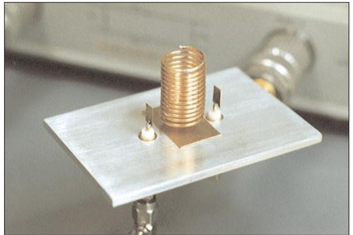
■ Figure 2. Vertically mounted solenoid in a transmission text fixture with capacitance coupling to the solenoid.
