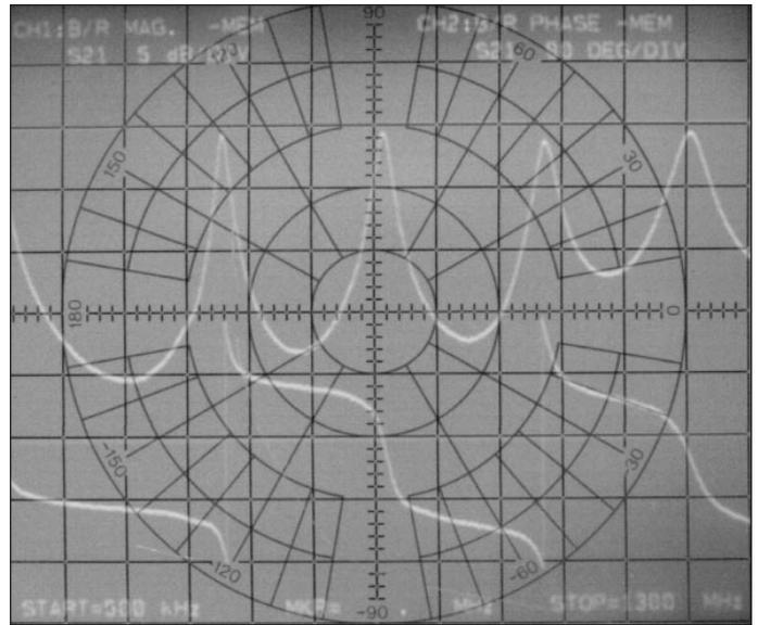
■ **Figure 5. Transmission amplitude and phase response of the horizontally mounted solenoid.**
