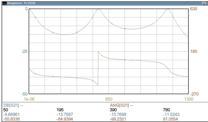
■ **Figure 11. Computer simulated transmission amplitude and phase responses of the transmission line model of the toroi plus 0.12 pF of parallel capacitance.**
