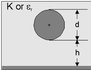
■ **Figure 8. Diagram of the wire over ground transmission line.**
