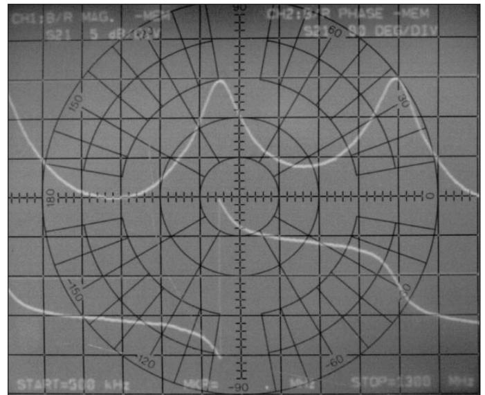
■ **Figure 10. Transmission amplitude and phase response of the toroid inductor.**
