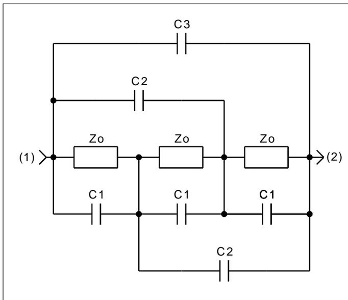
■ **Figure 20. Transmission line solenoid model, including interwinding capacitance typically required for solenoids with extreme diameter to length ratios.**
