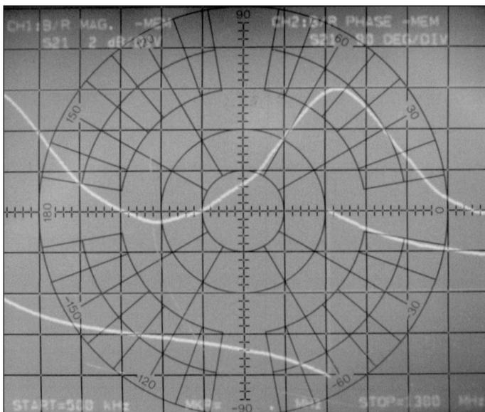
■ **Figure 16.** Measured transmission amplitude and phase response of the coaxial helical solenoid.
