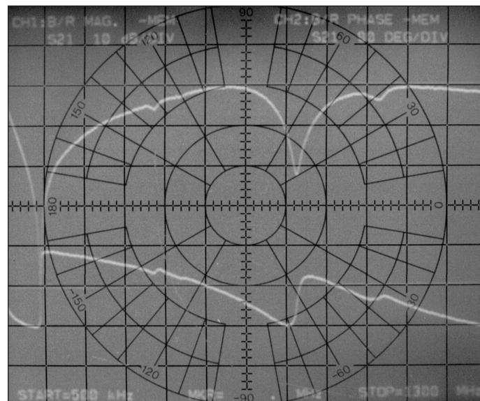
■ Figure 19. Measured transmission amplitude and phase response of the extreme diameter to length ratio solenoid.
