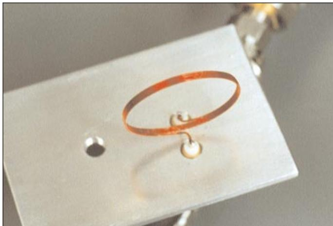
■ Figure 18. Solenoid with extreme diameter to length ratio, mounted in the transmission test fixture.
