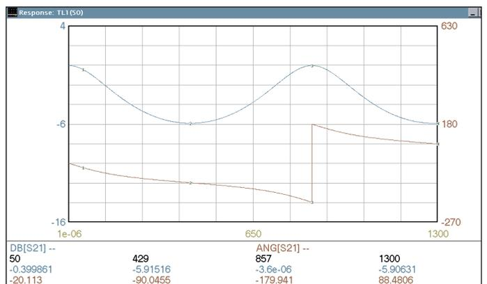
■ **Figure 17.** Computer simulated transmission amplitude and phase response of the transmission line model of the coaxial helical solenoid.
