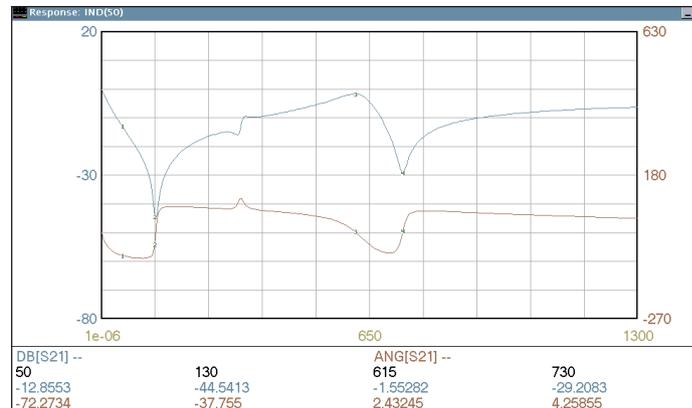
■ **Figure 21. Computer simulated transmission amplitude and phase responses of the model in Figure 20.**
