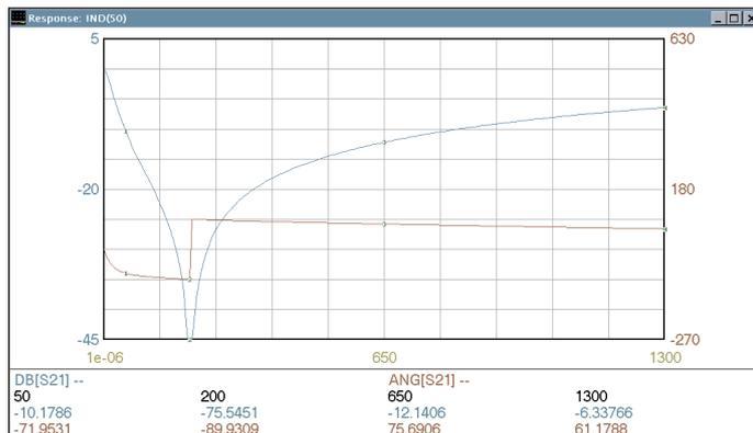
■ **Figure 6. Computer simulated transmission amplitude and phase response of the classic model of the solenoid shown in Figure 4.**
