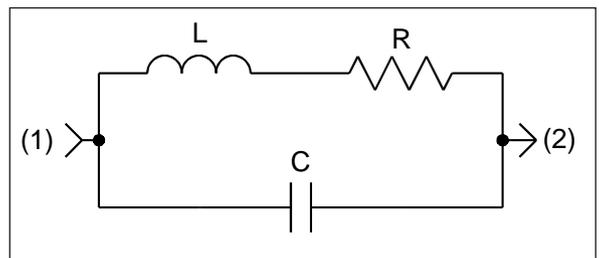
■ Figure 1. Schematic diagram of the classic inductor model.
