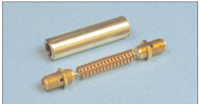
■ **Figure 15.** The coaxial helical solenoid, removed from its shield.
