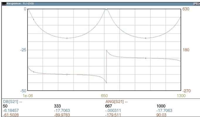
■ **Figure 14.** Computer simulated amplitude and phase response of the proposed transmission line model of the Coilcraft 132-20SM mounted over FR-4 substrate.
