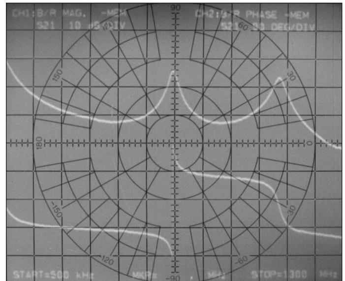
■ **Figure 13. Transmission amplitude and phase response of the Coilcraft 132-20SM mounted on an FR4 substrate.**
