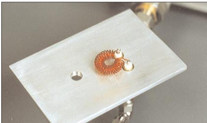
■ **Figure 9. Toroid inductor mounted in the transmission test fixture.**
