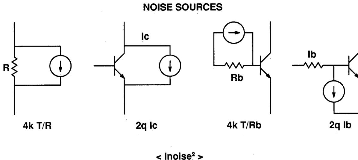
Figure 3. Noise sources for the active bipolar mixer.
