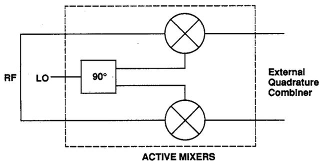
Figure 6. Circuit for an IC image rejecting mixer.
