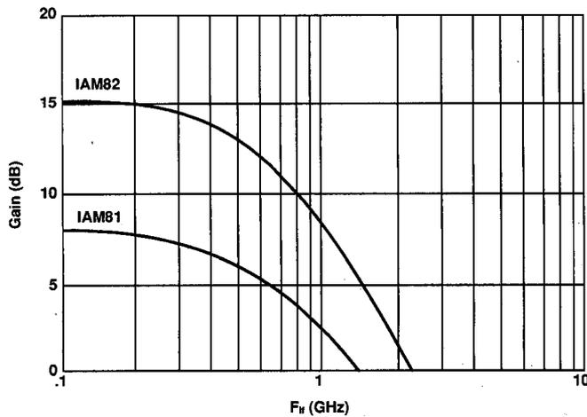
Figure 4b. Conversion Gain versus IF frequency, swept LO, RF = 2GHz.
