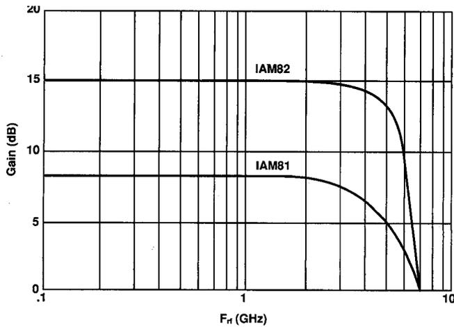
Figure 4a. Conversion gain versus RF frequency; swept RF and LO, IF = 70 MHz. Conversion gain is defined as the ratio of output power at the desired output frequency to the RF input power level, with the LO input at a stated value (-5 dBm for the IAM81, 0 dBm for the IAM82 – which are the LO input levels for which the devices are designed).
