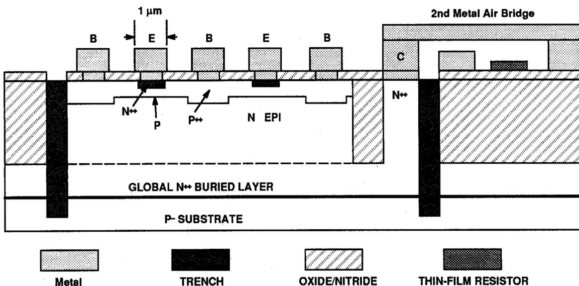
Figure 1. Cross section of the isolated self aligned transistor process.
