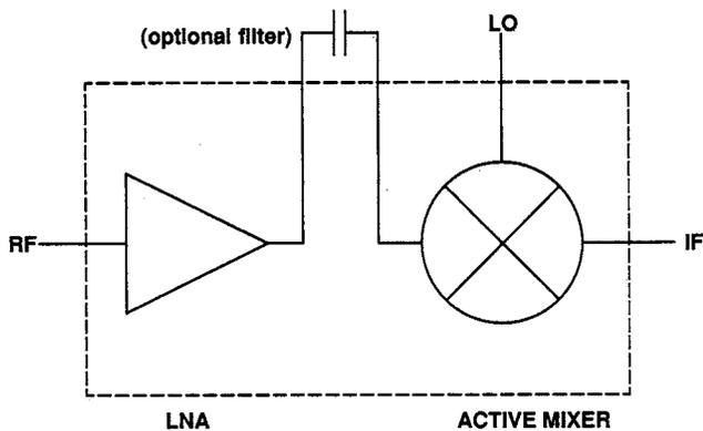
Figure 5. A low noise active mixer IC.
