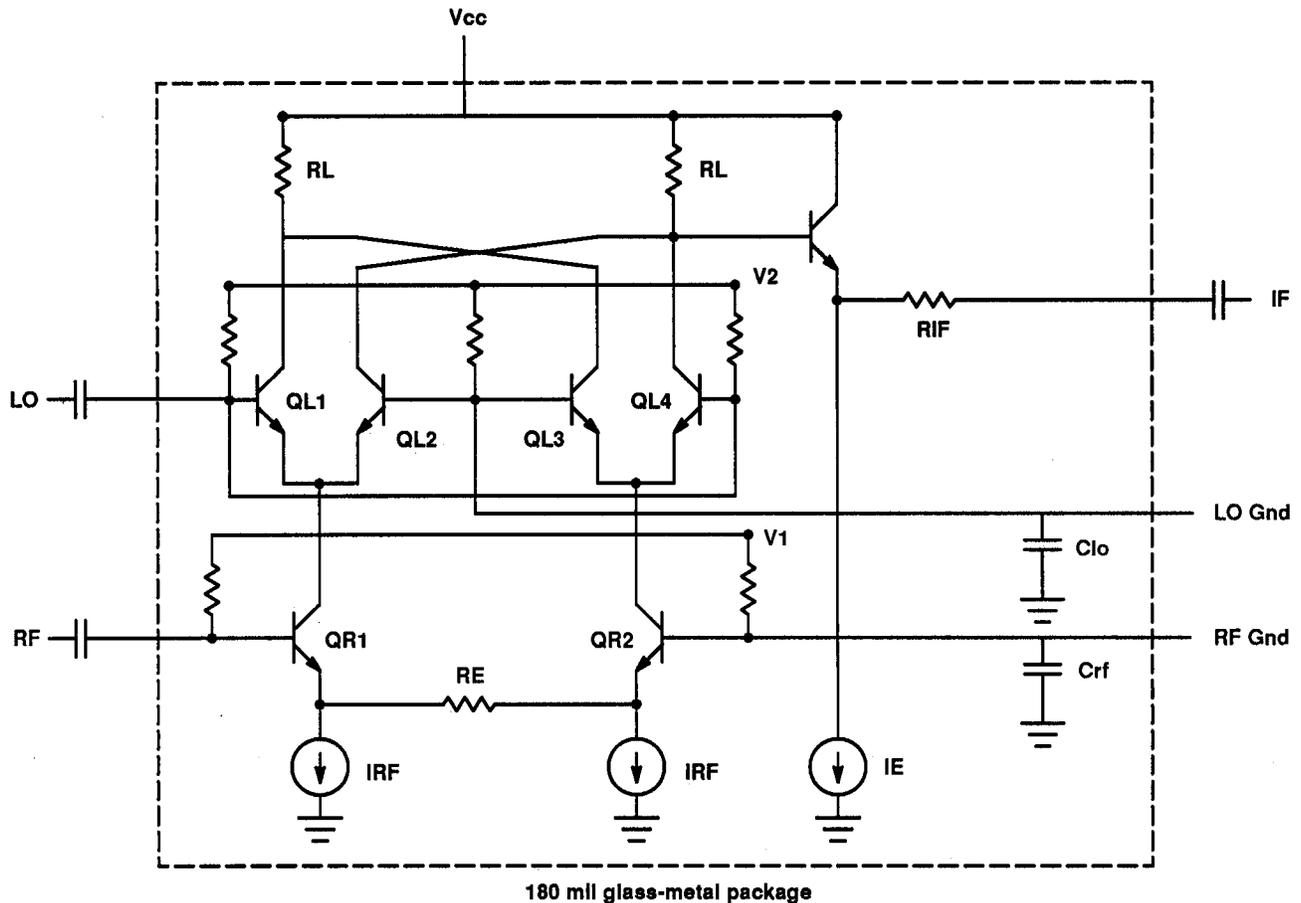
**Figure 2. Simplified schematic of the active bipolar mixer.**
